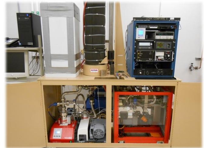
Std. Chamber (left) and UUT Chamber (right). Underneath, ULTRATEST F leak detector on right, modern counterflow leak detector and backing pump on left.
