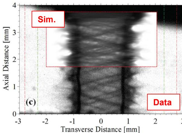
Radiograph from T. J. Awe *et al.*, *Phys. Plasmas*, **21**, 056303 (2014) showing the modified MRT structure in flight along with synthetic radiograph from a GORGON calculation (inset).
