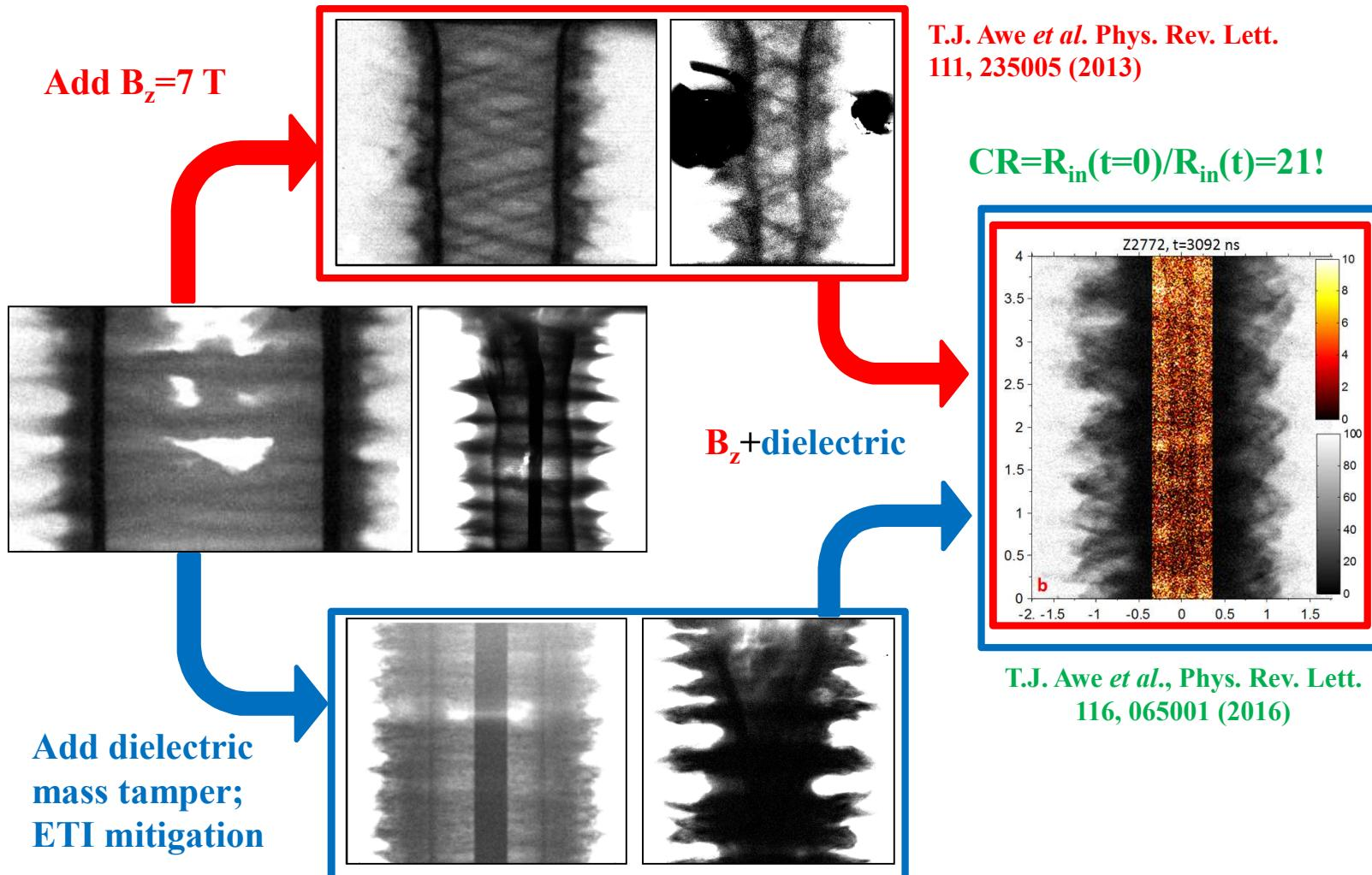
**Employing coated liners in a recent integrated experiment has demonstrated improved symmetry and reduced mix**
