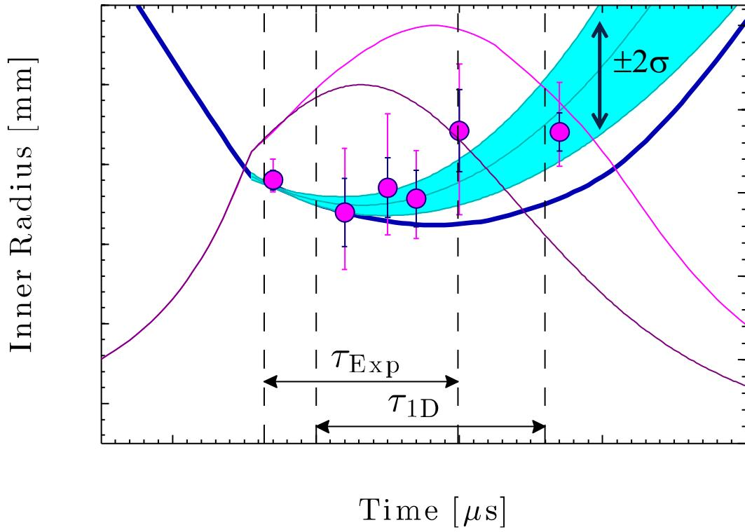
Blue interval is the  $2\sigma$  interval fitting the data, including a  $\pm 1$  ns uncertainty in radiograph timing
