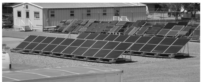
Fig. 1. The present work performed tests on a 10.8kW e array. The array has four strings that each have 10 modules. The strings are combined prior to entering the inverter. In addition, each of the string's current and voltage are monitored.
