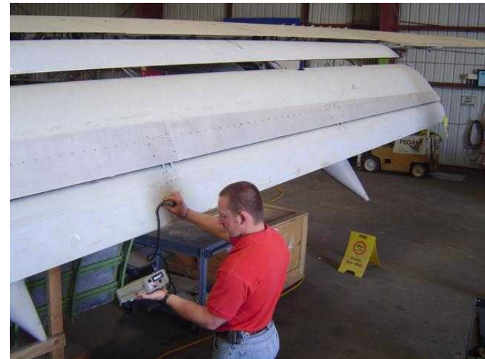
Aircraft ultrasonic inspection (Composites World)
