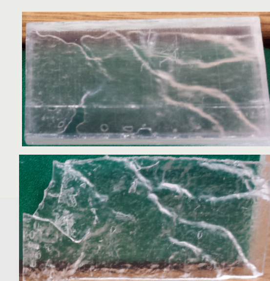
3D printed single fracture network (top) and fracture aperture (bottom)
