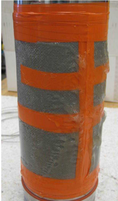
Fig. 2. Specimen with end caps and wrapped in the steel frit material. The orange electrical tape is used to close the frit around the specimen and to connect the specimen, end cap and frit together. This whole assembly is then jacketed in viton in the case of the granite or polyolefin in the case of the shale.
