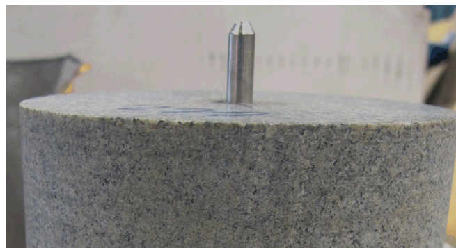
Fig. 1. Image of the casing pipe epoxied into place in the center of a specimen. The pipe extends beyond the top of the specimen in order to seal with the endcap, and the bottom 1.9 cm of the hole was left uncased.
