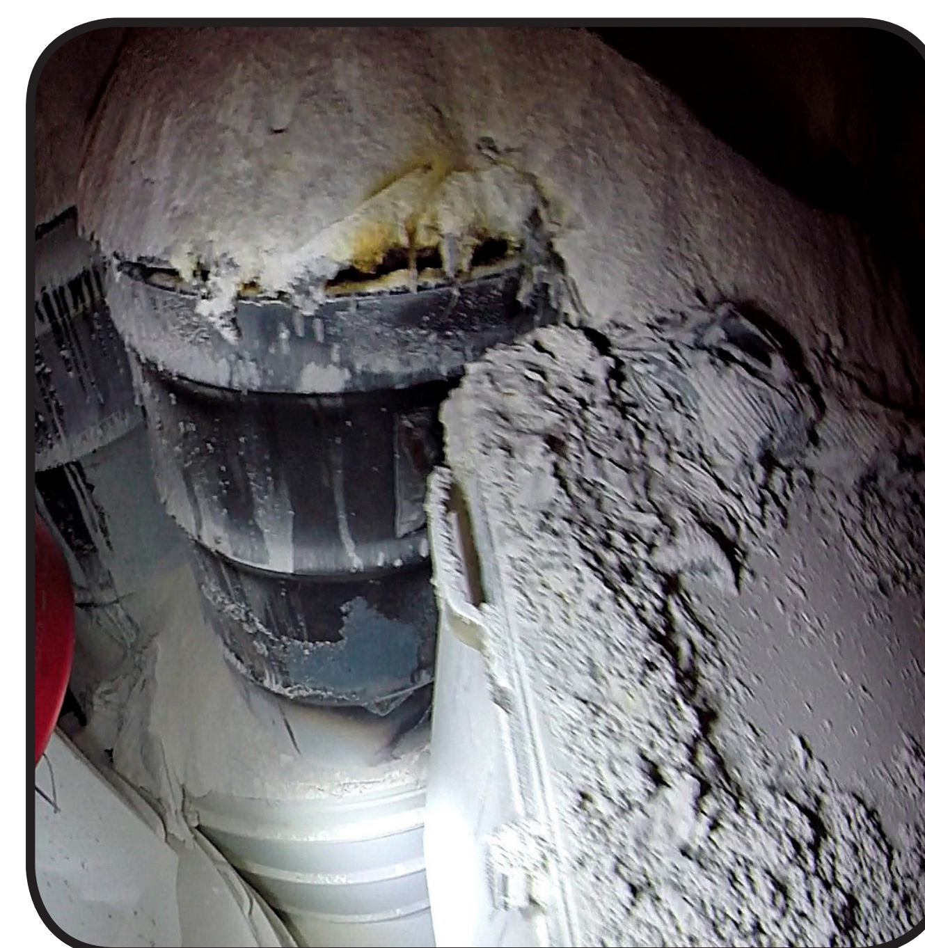
TRU Waste Drum 68660, the drum in Room 7 of Panel 7 at WIPP known to have breached.
