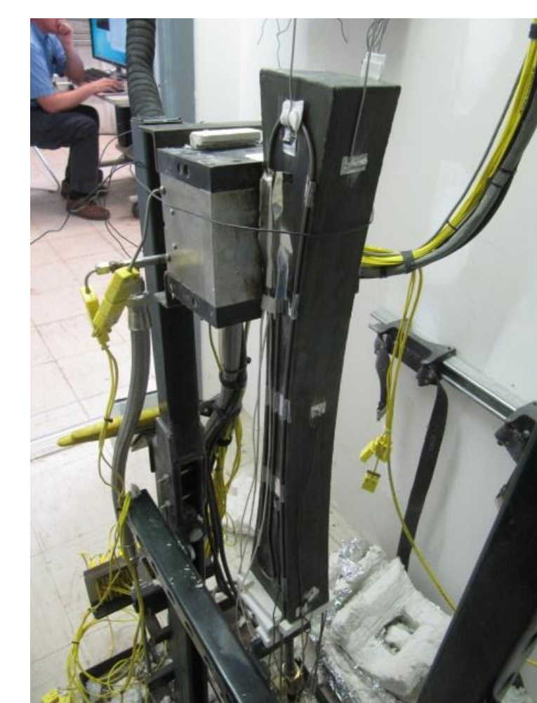
Bench-scale heat pipe durability test rig
