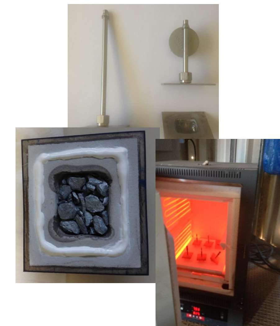
Air furnace and closed boat assembly
