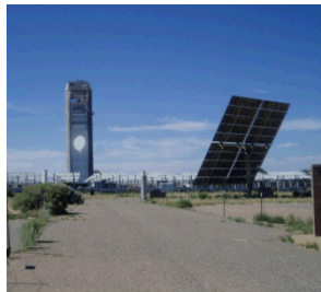
Full-scale heliostat modeling and testing at the NSTTF
