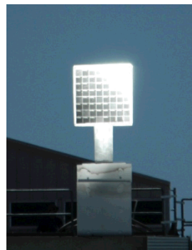
Shuttle Tile Testing on top of Solar Tower
