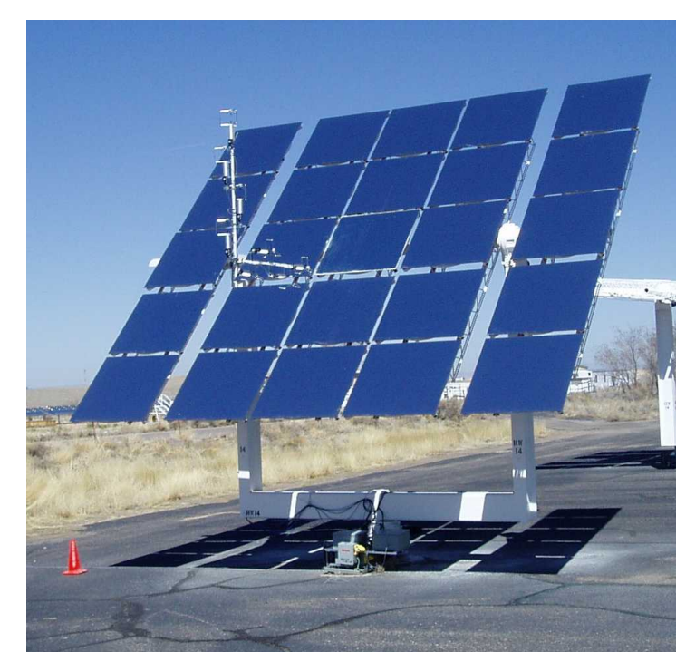
Full-scale heliostat testing at the NSTTF enables validation of models and design tools
