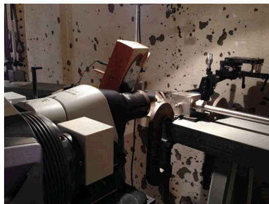
Experimental configuration for 1 MHz DIC of a closure disk
