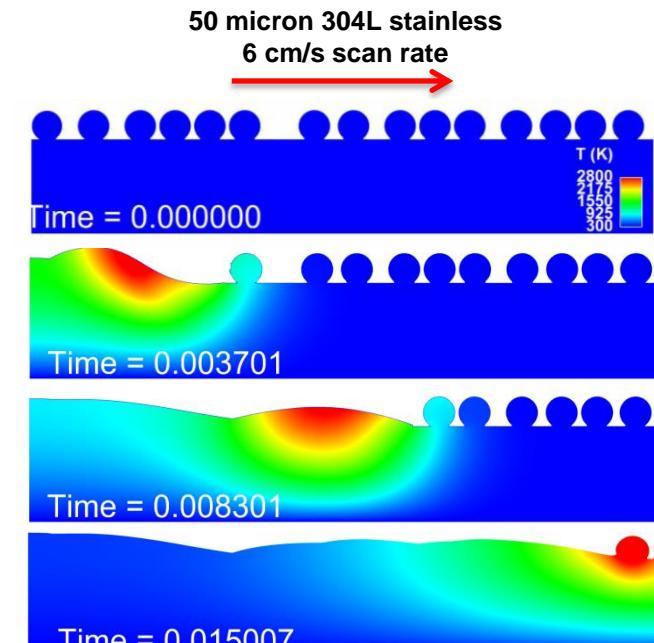
Additive Manufacturing via selective laser melting
