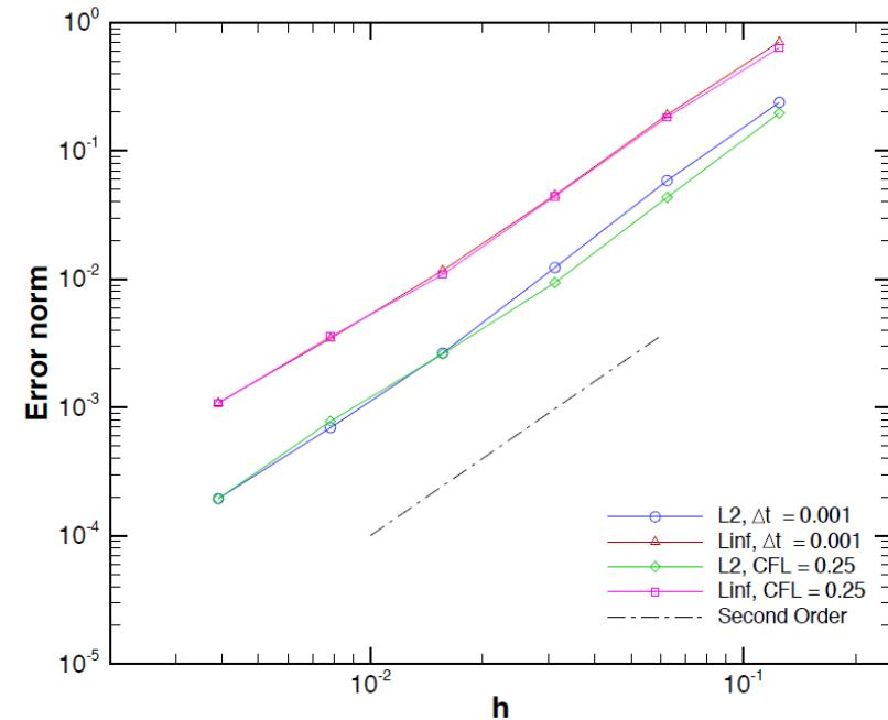
Convergence plot for the 2-D advection-diffusion problem with contact resistance, using the BDF2 time integrator
