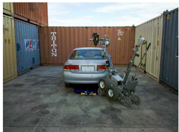
EOD Robot using X-ray scanner to X-ray vehicle contents during an exercise
