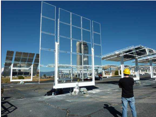
Heliostat with 3M™ Solar Mirror Film 1100
