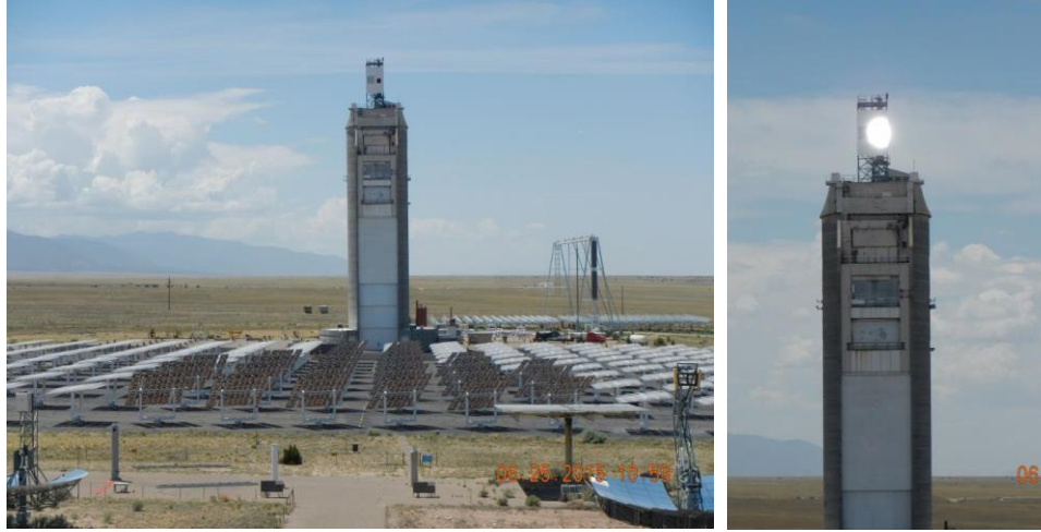
FIGURE 3. On-sun testing of the particle receiver prototype at the top of the tower. Left: heliostats in standby position. Right: heliostats aimed at receiver.
