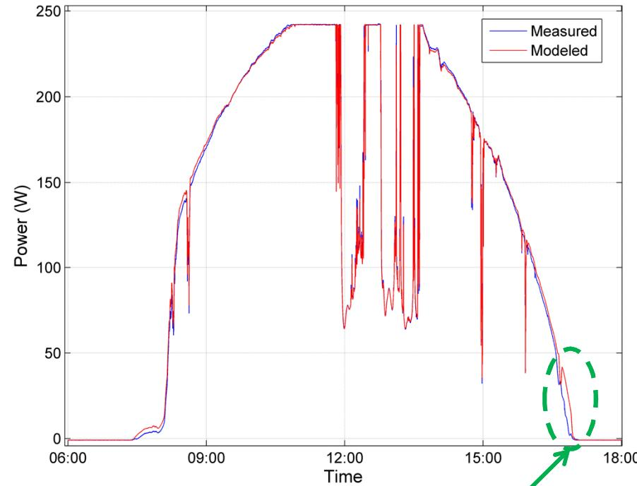
Shading of the module but not the irradiance sensor. Data omitted from subsequent analyses.
