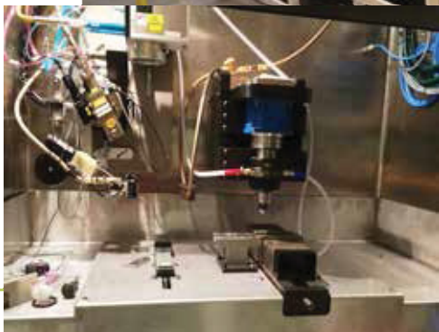
The welding cubicle, enabling development and testing of advanced welding techniques on irradiated materials, is lowered into the hot cell. The friction stir weld system (inset photo) was successfully tested.
