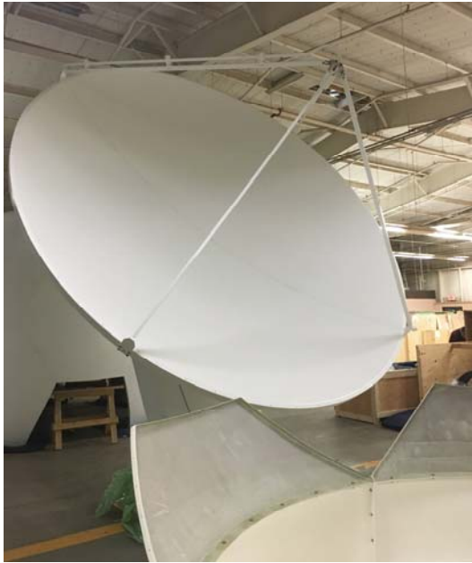
Figure 10. Struts and feedhorn installation on the front side of the antenna. Waveguide and supporting brackets were installed down the strut.
