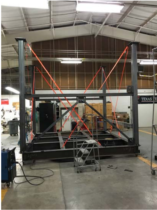
Figure 12. Exoskeleton support platform.
