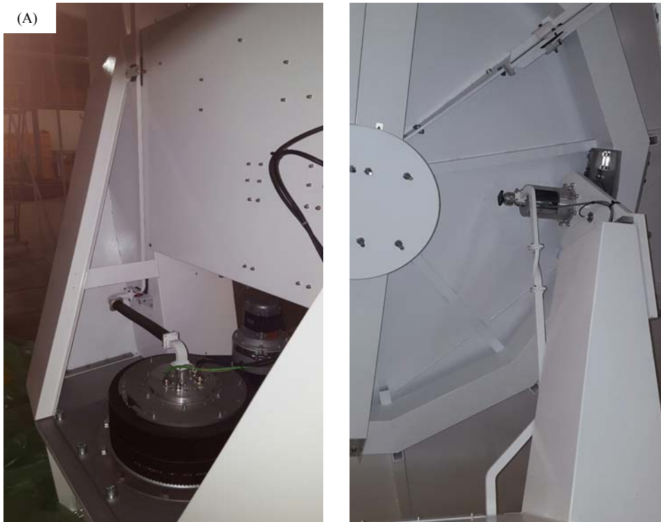
Figure 9. Azimuthal (A) and elevation (B) rotary joints installed on the antenna/pedestal subsystem.
