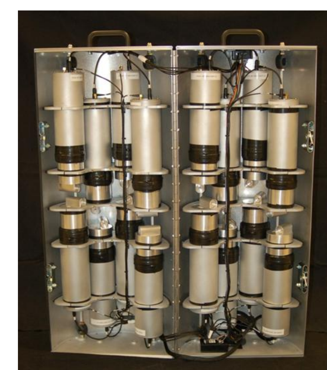
Fig. 4. MINER system (left) and measurement setup (right) of the two Cf-252 sources measured.
