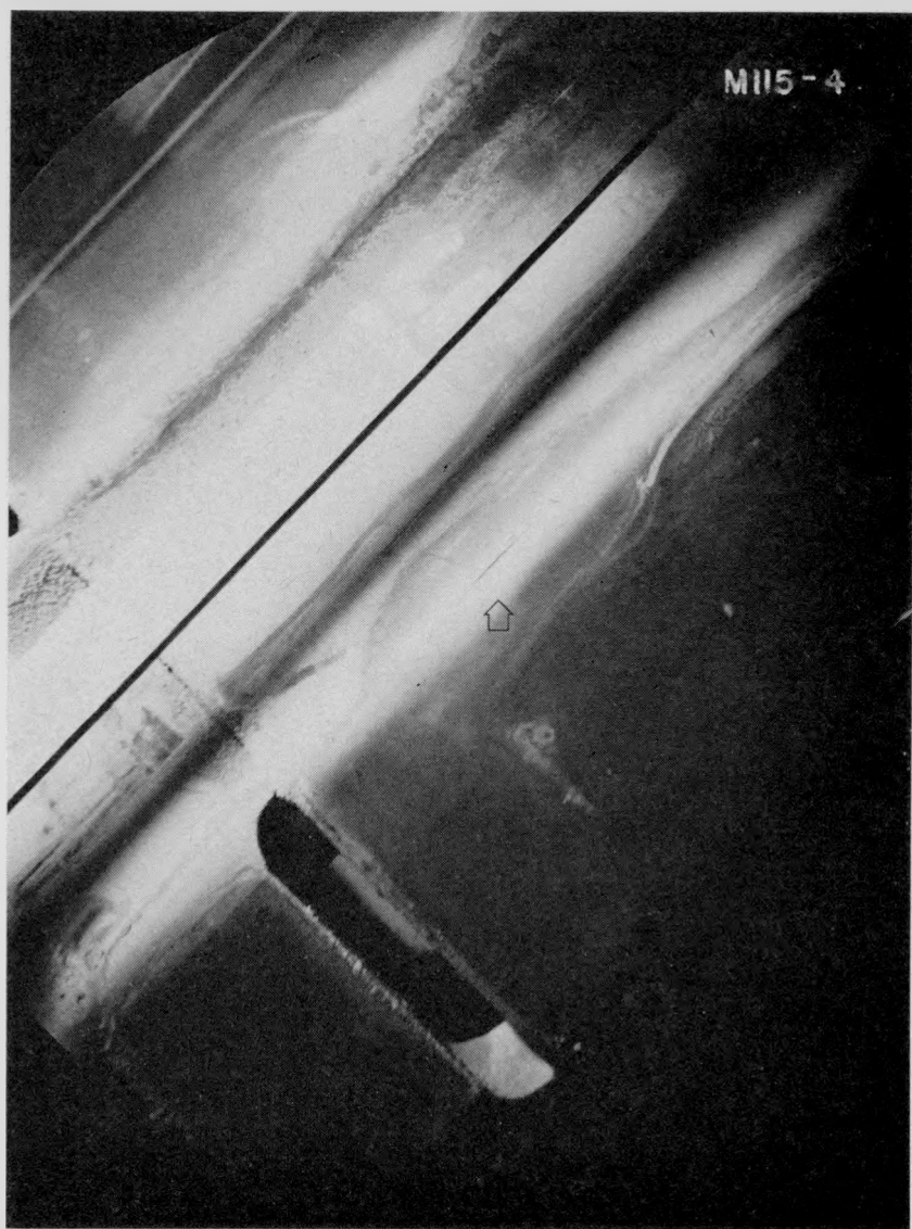
Moderator Can Crack. Photo shows a typical crack (indicated by arrow) of the type found in 19 of the moderator cans of the Hallam, Nebr., sodium-cooled reactor. It was through such cracks in the stainless steel sheaths of the 17-foot-long moderator cans that the molten sodium penetrated and caused the moderating graphite to swell. The contract for operation of the reactor was terminated in mid-1965. The reactor had been shut down in September 1964, when it was believed only seven of the cans had cracks.
