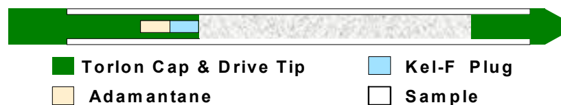
Figure 1. Schematic representation of the rotor assembly with the adamantane-packed cap (adamcap) used in quantitative coverage assessments of ceria nanocubes.
