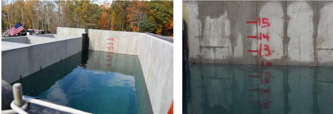
Figure 9 – Test Tank with 12' retained water
