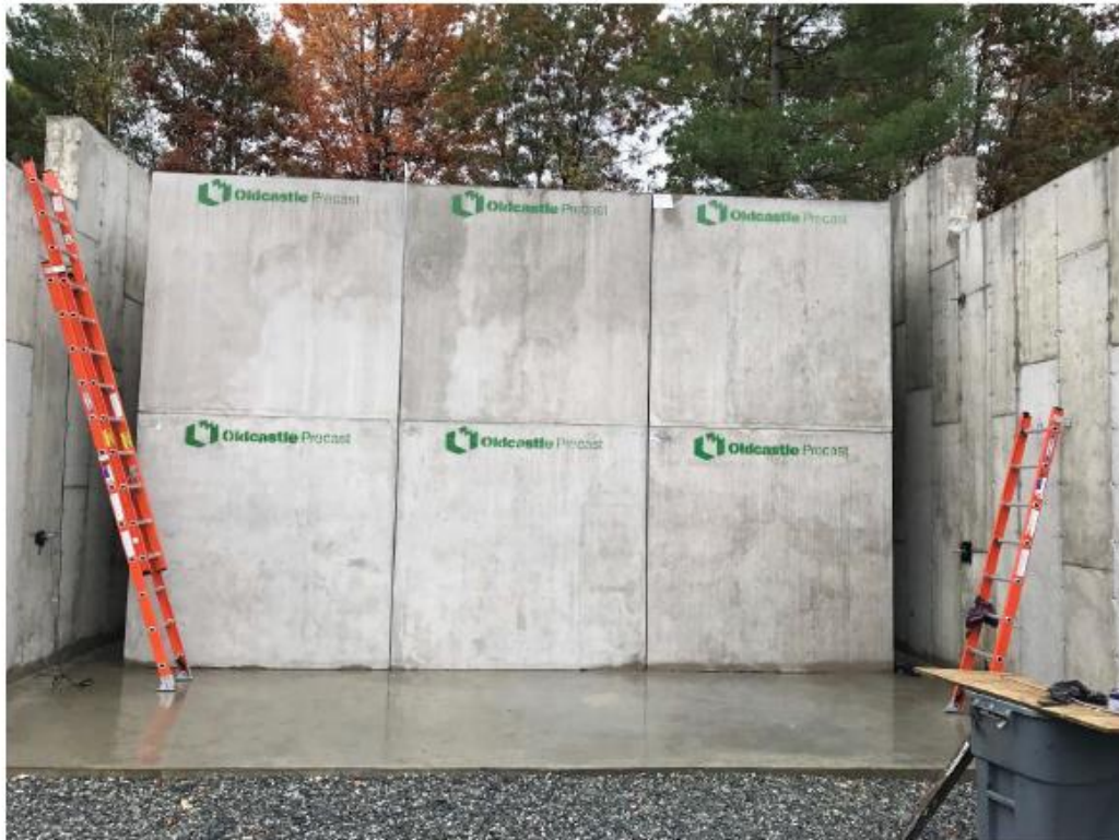
Photo 4 – Water at a depth of 144 \frac{3}{8} inches taken at the manometer tube located on the left wall of the tank as you are looking upstream at the dam. There is a drip of water every 3 to 4 seconds leaking at the bulkheads. There is no sign of water downstream of the modular dam.
