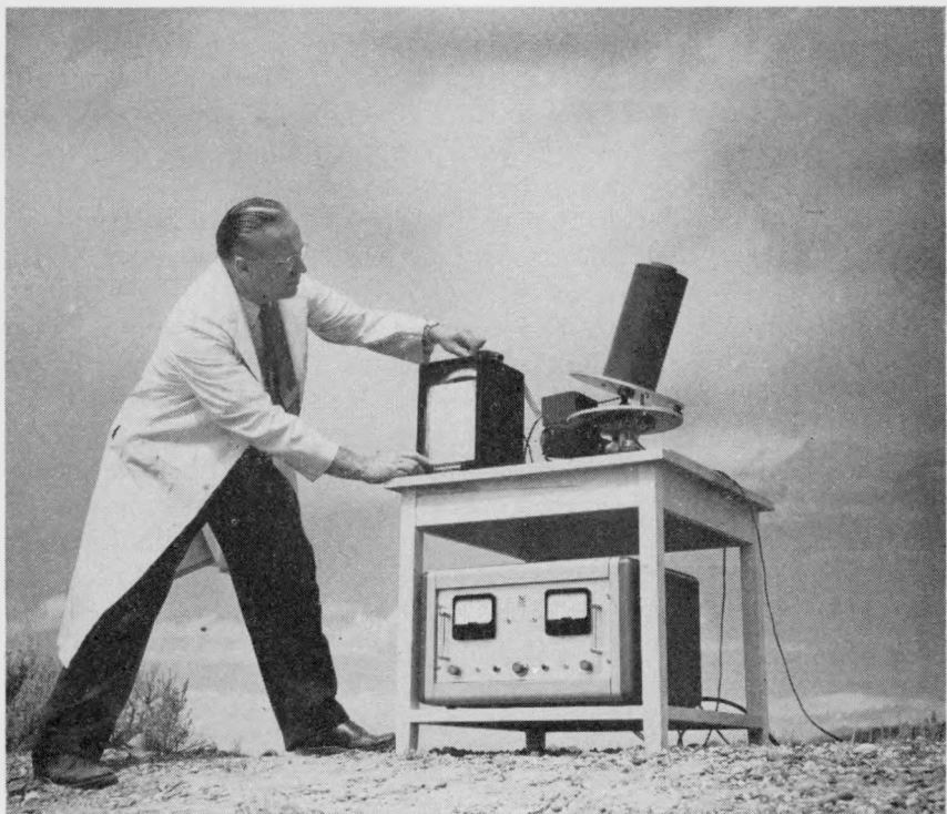
Sky scanner. An instrument developed by the Idaho Operations Office's Health and Safety Division is used to track radioactivity released from stacks at the National Reactor Testing Station.
