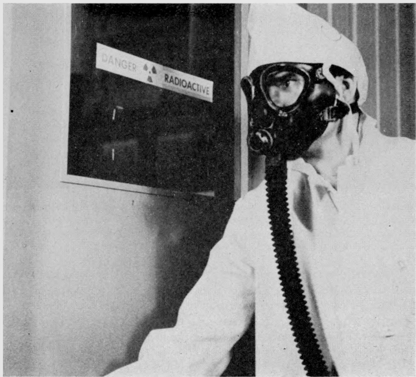
Entering a "cave". Dressed for protection against contamination in a "hot cave" at Mound Laboratory, Miamisburg, Ohio, the worker wears special, discardable clothing, rubber gloves, a mask with an independent supply of oxygen.
