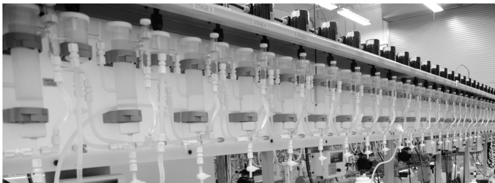
Figure 4 – Thirty stage mixer-settler system at the Idaho National Laboratory.
