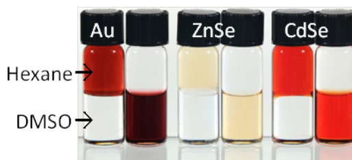
Fig. 3 (Left) Schematic of ligand exchange by treatment with \text{NH}_4\text{SCN} . (Right) Biphasic mixtures of hexane and DMSO with as-synthesized NCs on the left of each pair and NCs treated with \text{NH}_4\text{SCN} , washed, and re-dispersed in DMSO with hexane added on top on the right for: (left to right): Au, ZnSe, and CdSe NCs.
