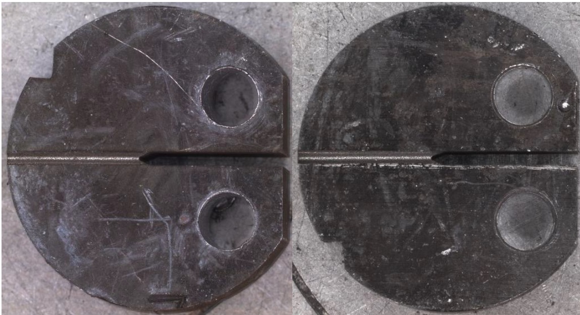
Figure 2-2: Image of sample RCT1 from both sides. It is clearly evident that a small amount of material was removed during the fabrication of tensile sample T3; however, this should not significantly affect the stress intensity during the CGR test.
