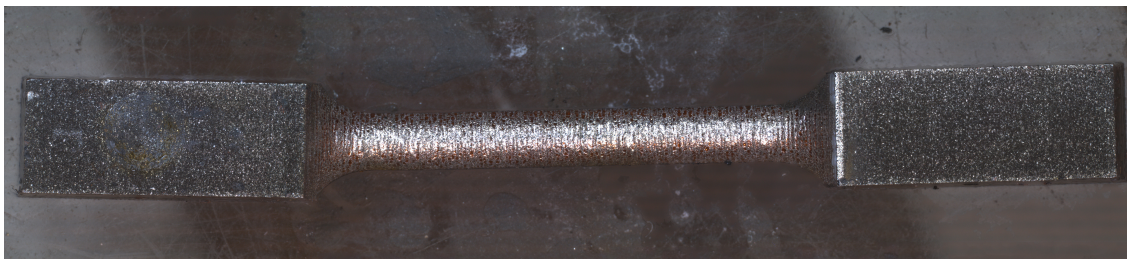
Figure 2-4: Side view of sample T5, which was likely deformed during the handling of the sample post-fabrication.
