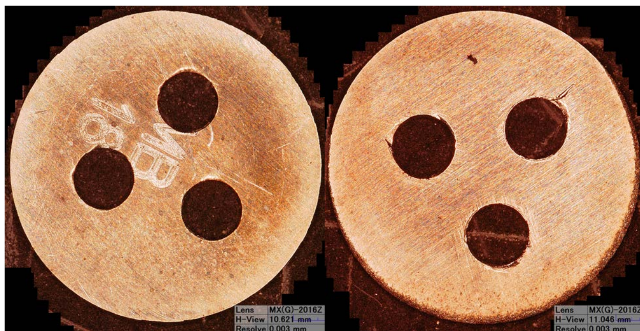
Figure 6. MA956 Irradiated DMC, MB-18 from capsule 5-2 400c, 6.2 dpa. Sample is 8mm diameter imaged at 20x, and the top is seen in the left image, bottom at the right. Cracking can be seen around the punch holes in the right image.
