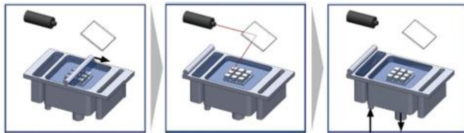
Figure 1: Three-step SLS process which involves, from the left, the rolling of the powder material across the bed, the laser sintering of the powder, and the lowering of the bed to allow the next layer to roll over the sintered layer. 2
