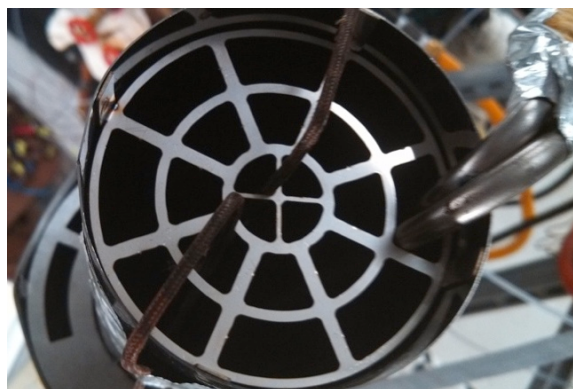
Figure A2. Detailed image of temperature probes and emissions sampling probes for Rheem RTG-84DVLN. Emissions was sampled 12-inches into the exhaust vent. Exhaust temperature was measured 12-inches into the exhaust vent in two locations.
