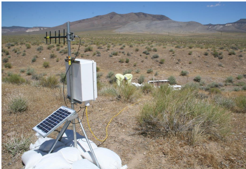
Figure 5. Runoff conditions in the flume are detected by the pressure transducer (yellow cable), recorded in the datalogger (white box), and relayed by radio (black antenna) to the meteorological station for transmission to the Western Regional Climate Center via GOES satellite.
