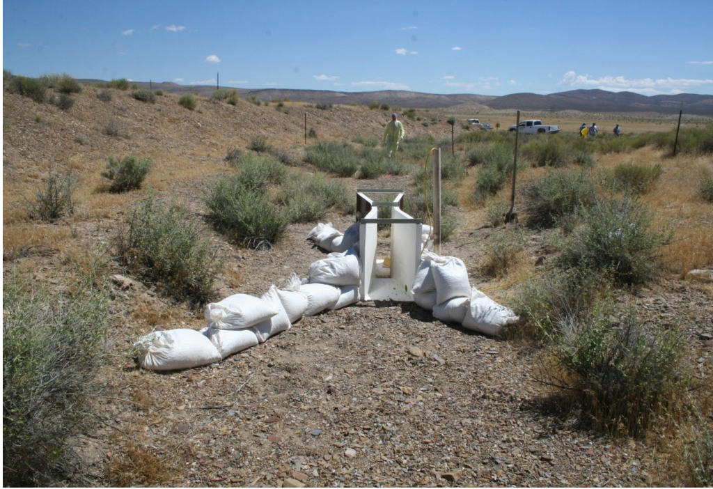
Figure 4. View looking downstream through the flume installed to measure runoff from the Smoky CA (prior to washout in July 2013).
