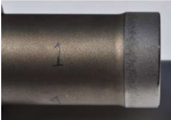
Figure 31. HT piston wear progression (stem end)
