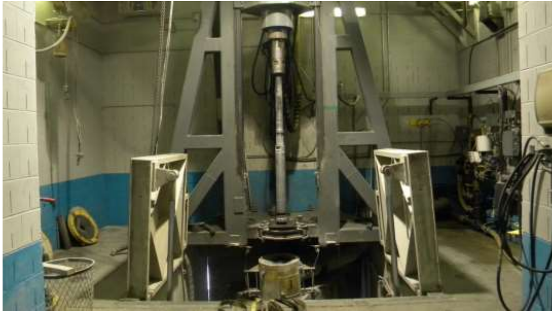
Figure 11. Drill Tower, Showing Basement Access for Rock Sample
