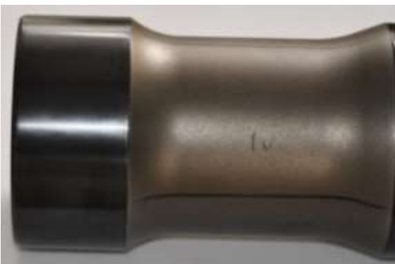
Figure 41. LT piston visual wear after 25.5 ft
