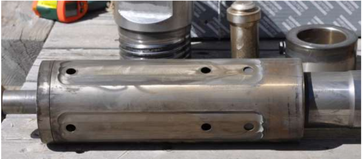
Figure 23. Piston sleeve assembly after operating at 400°F
