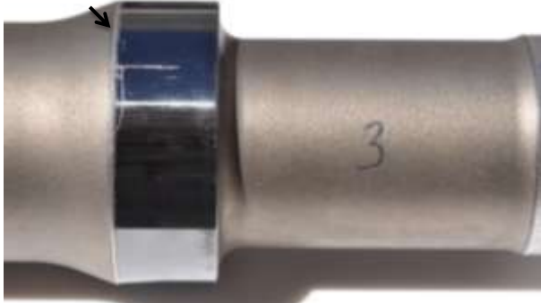
Figure 32. HT piston wear progression (mid-section)
