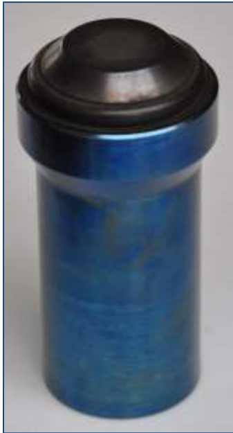
Figure 47. Check valve tempering temperature color change
