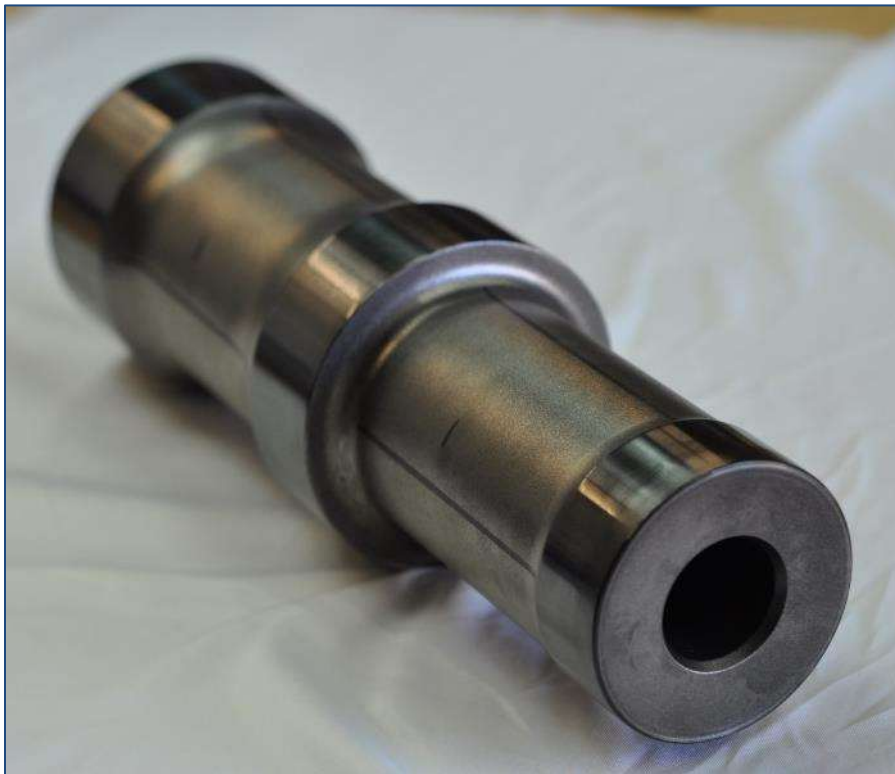
Figure 35. LT piston with DLC coating applied
