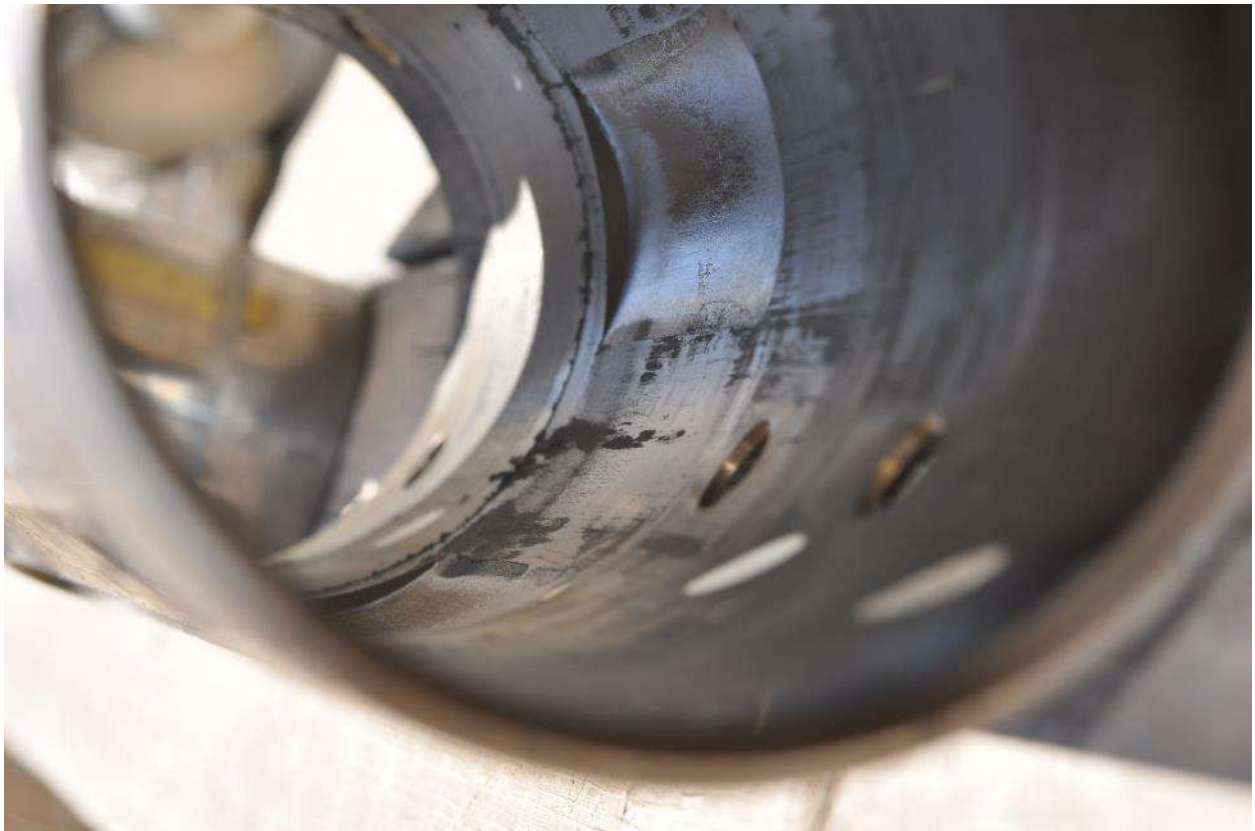
Figure 24. Piston sleeve inner diameter after operating at 400°F
