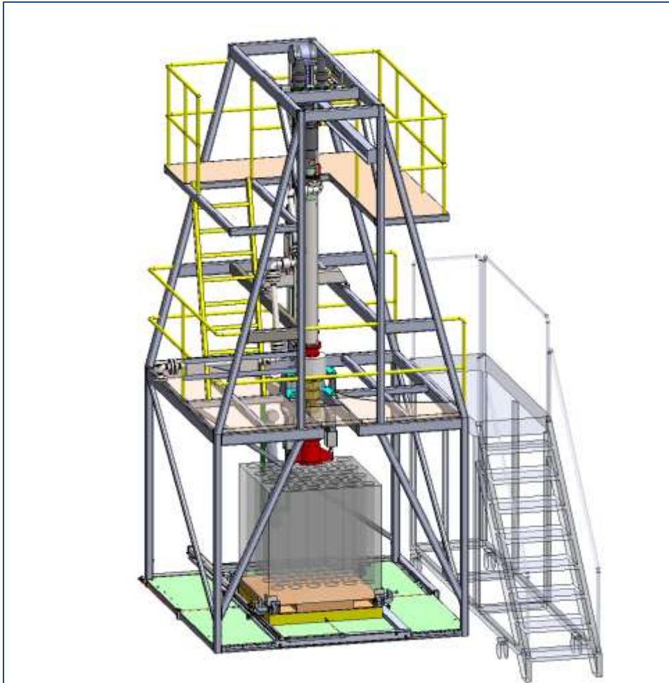
Figure 68. HOT test cell drill structure solid model
