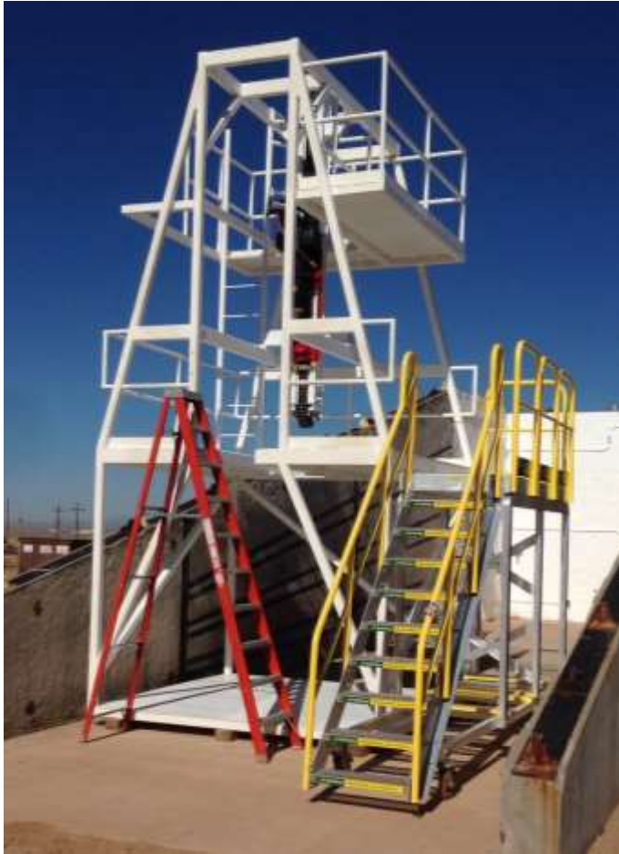
Figure 69. HOT test cell drill structure frame as built
