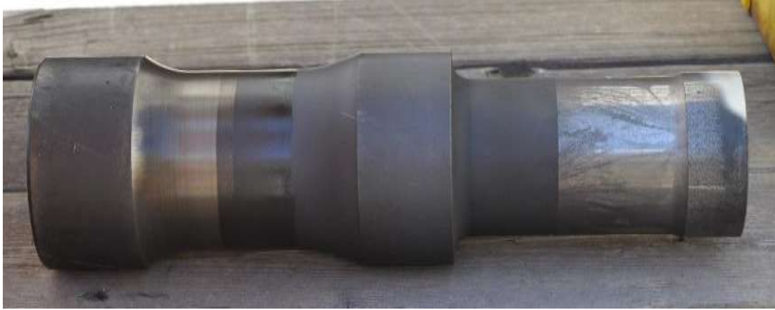
Figure 25. Piston with no lubrication at 400°F
