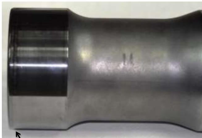
Figure 43. LT piston with DLC performance after 79.5 ft
