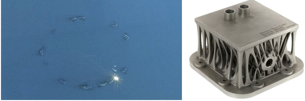
FIGURE 1.1. Left: Photo of the selective laser melting process [77]. Right: Complex manifold produced with a 3D SLM printer [1].
