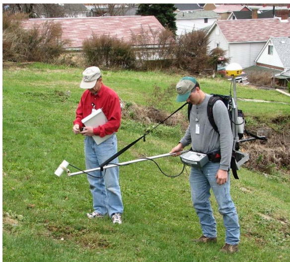
Figure 4: Magnetic surveys were conducted using a Geometrics 858 magnetometer with GPS.
