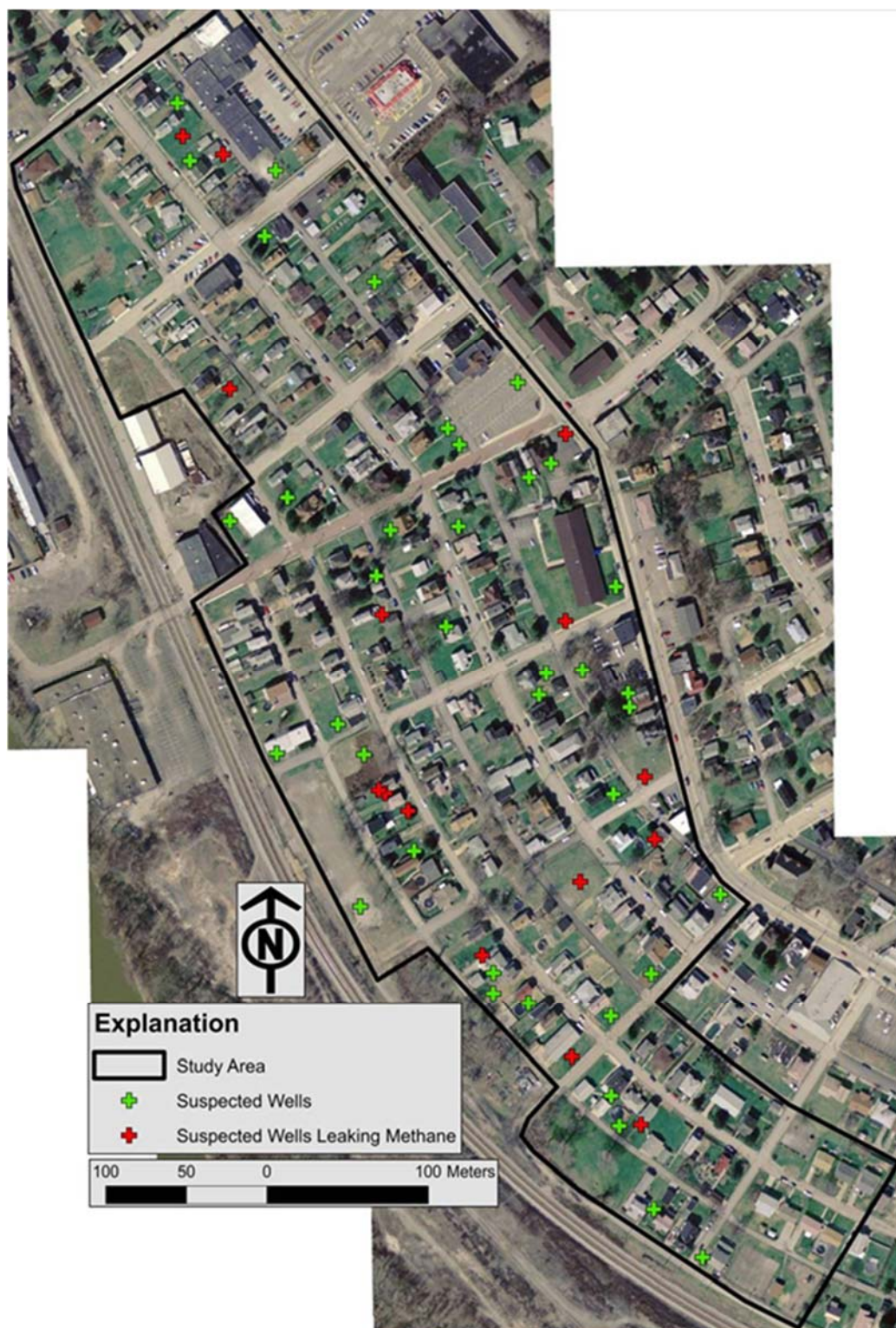
Figure 9: Google Earth image of Versailles Borough showing the locations of well-type magnetic anomalies (+) and well-type magnetic anomalies with anomalous CH 4 concentrations (+).
