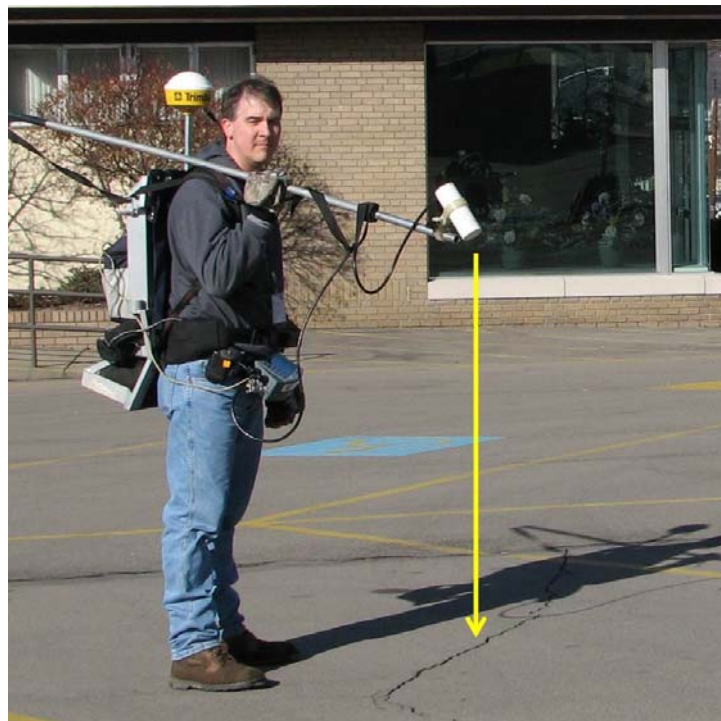
Figure 11: Magnetic survey indicates that a well is located beneath this parking lot (yellow arrow). There was no corresponding CH 4 anomaly.
