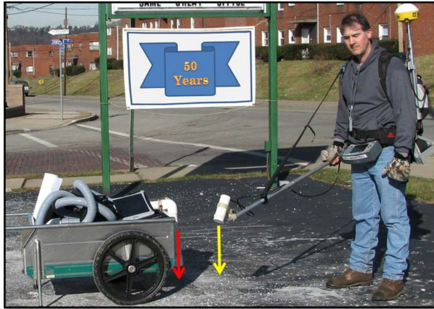
Figure 10: Leaking gas well underlies this paved lot. Red arrow shows location of maximum CH 4 concentration; magnetic sensor (yellow arrow) shows location of magnetic maximum.
