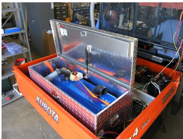
Figure 3: Apogee LDS sensor mounted in bed of 4-wheel drive utility vehicle.
