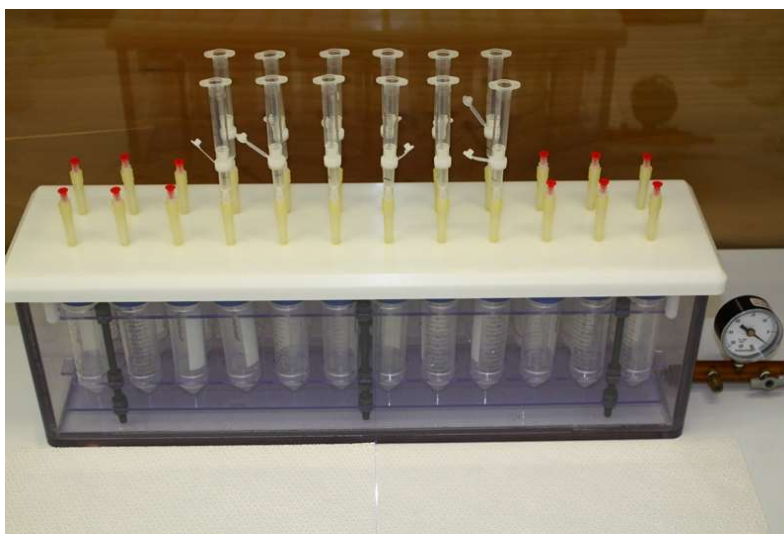
Figure 3: Vacuum box for Sr separation chemistry. The box can accommodate up to 24 samples per batch.
