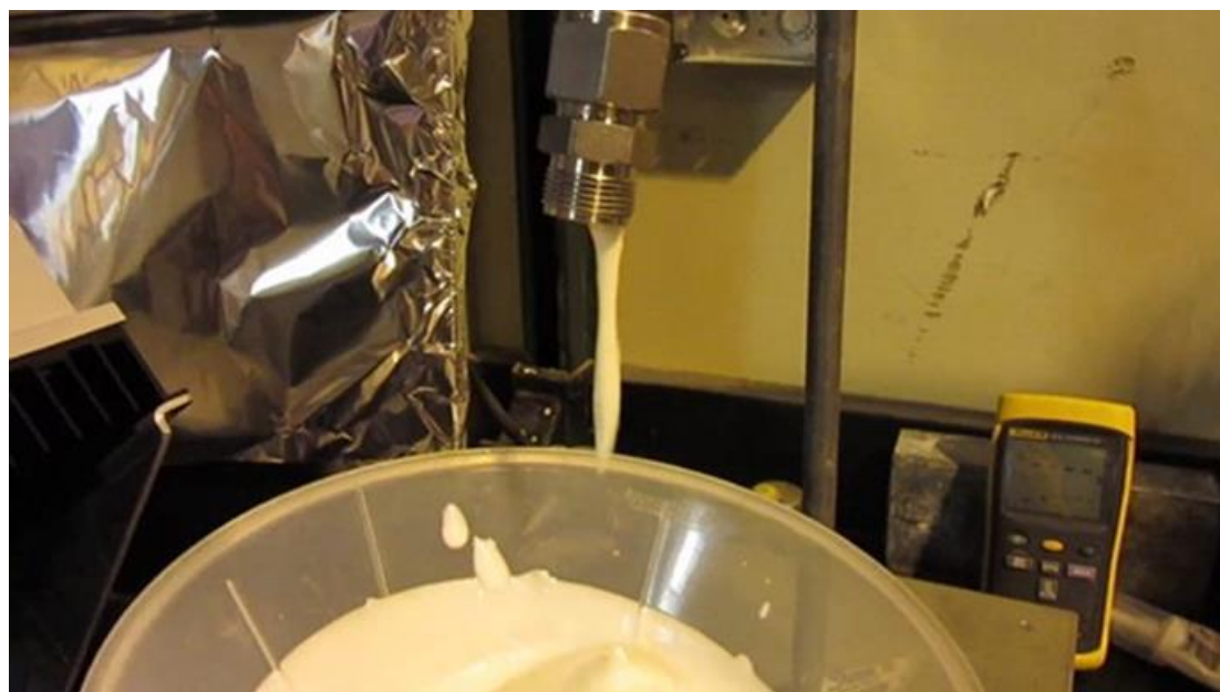
Figure 55. Pumping of 56.7% carbamate slurry into inlet funnel.
