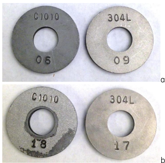
Figure 41. Carbon steel and stainless steel coupons after 6 weeks of exposure to a) control conditions and b) desorber conditions.
