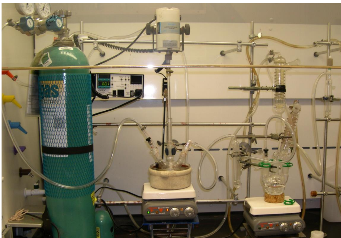
Figure 77. SO 2 Gas Absorption Apparatus.
