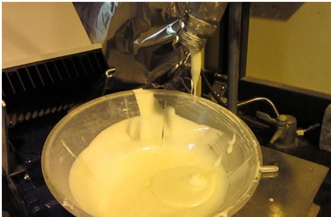
Figure 56. Pumping of 66.2% carbamate slurry into inlet funnel.
