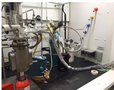
FTIR and Gas Delivery system
