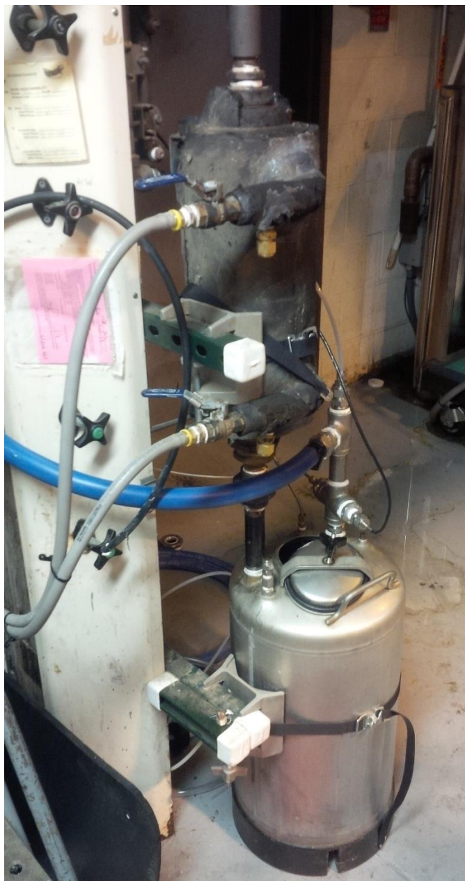
Figure 75. Heat exchanger added to absorber gas exhaust line.
