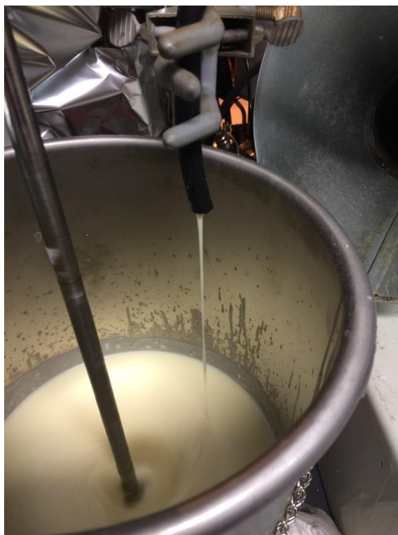
Figure 66. Slurry holding tank having continuous agitation.
