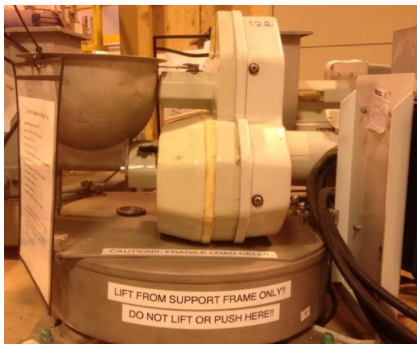
Figure 6. K-Tron feeder for supplying carbamate solids to WP ZSK25 extruder.
