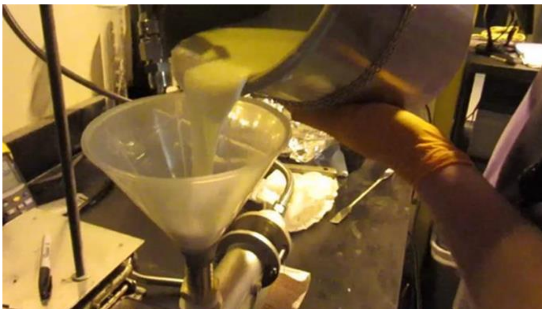
Figure 54. 56.7% carbamate slurry being poured into funnel at pump inlet.
