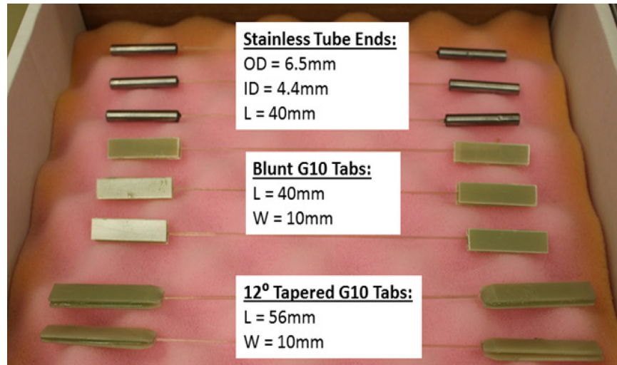
Figure 8 Early evaluation of other tapping methods for stress rupture test setup
