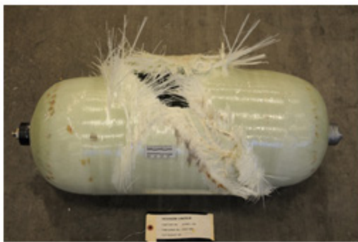
(e) COVP E-Glass: 79% load for 3 min (f) COVP E-Glass: 922 cycles
