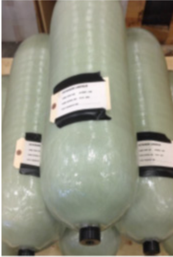
(a) COPV A-I STEB 250 bar (b) COPV A-I: Post 45,000 Cycles & Post Cycle Burst (10.6 KSI)
