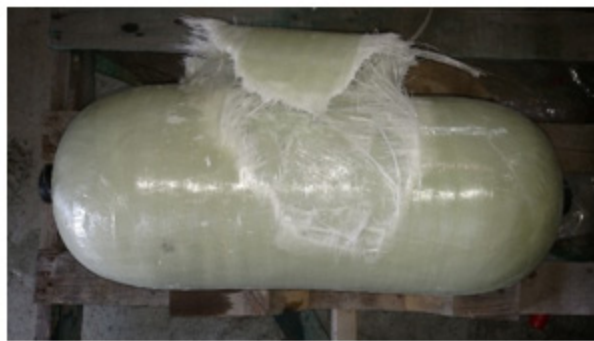
(e) COVP E-Glass: 79% load for 3 min (f) COVP E-Glass: 922 cycles
