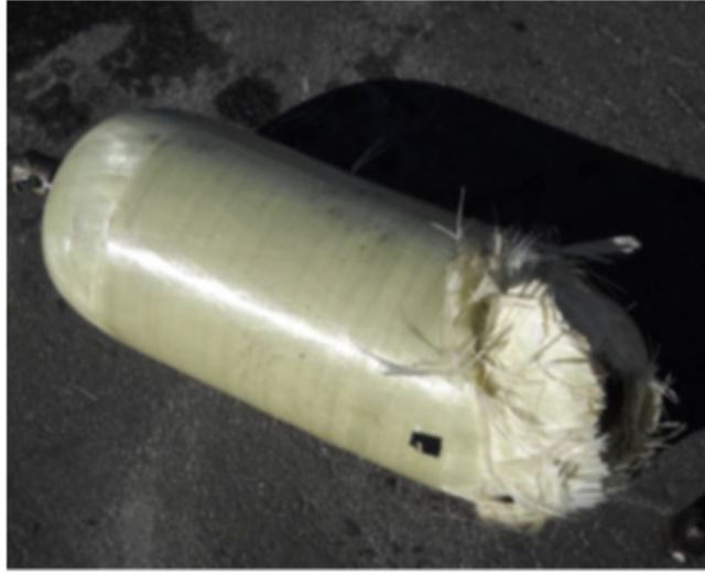
(a) COPV A-I STEB 250 bar (b) COPV A-I: Post 45,000 Cycles & Post Cycle Burst (10.6 KSI)
