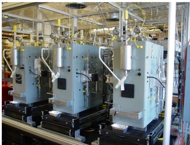
Figure 12. Laboratory-scale microreactor systems for WGS testing
