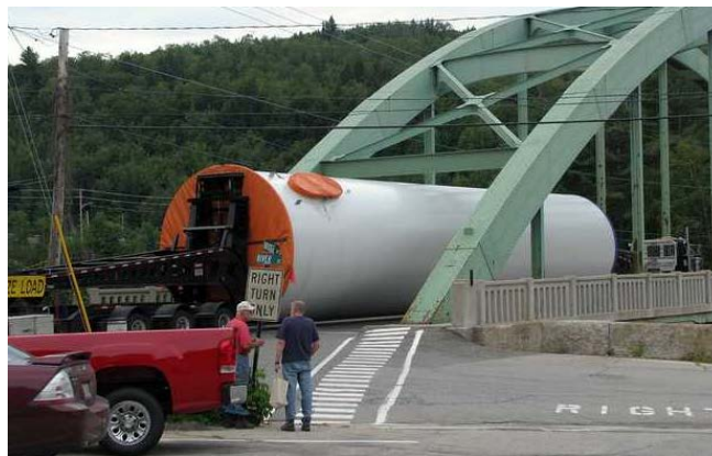
Figure 2.2. Challenge in transport of traditional steel tubular towers (Sun Journal, 2012)
