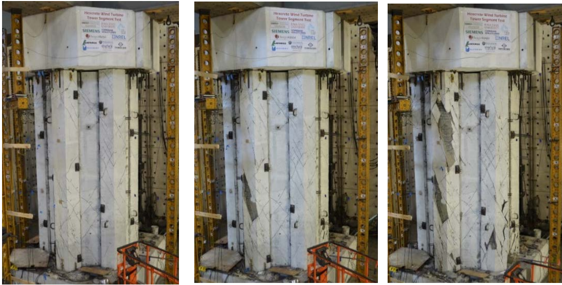
Figure 1.7. Damage progression of test unit under large displacement loading
