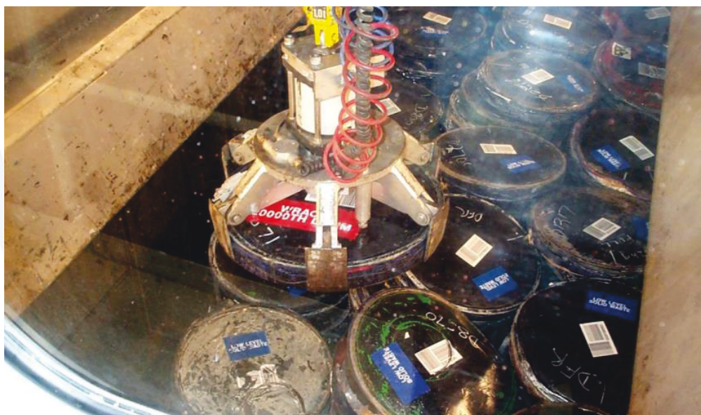
Figure 18. Photograph of a Super Compacted Drum (puck) Being Loaded in to an ISO-Freight Container in the Dounreay Waste Receipt Assay Characterization and Super Compaction Facility (WRACS) (Ref 252).
