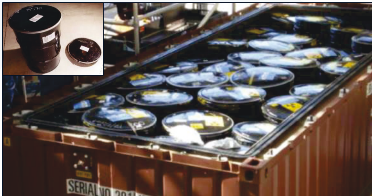
Figure 10. Supercompaction of LLW Drums into 'pucks' and Placement in a Half-Height ISO Freight.
