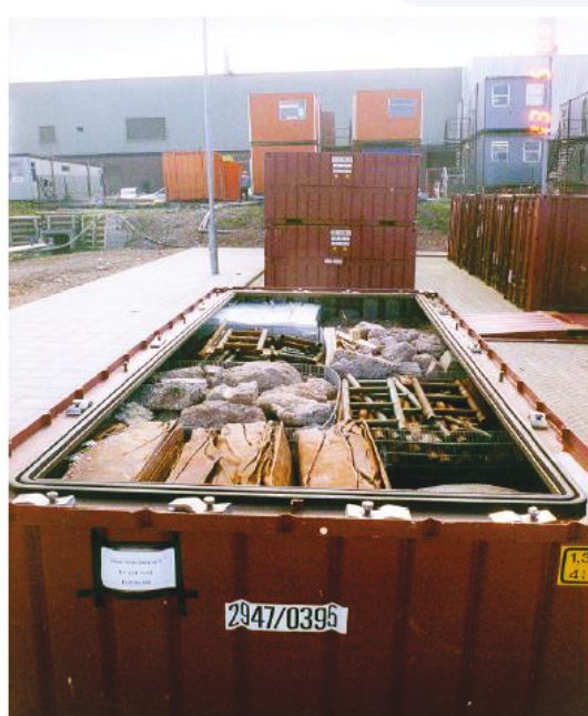
Figure 11. View of Demonstration ISO Prior To Grouting (Ref 246).
