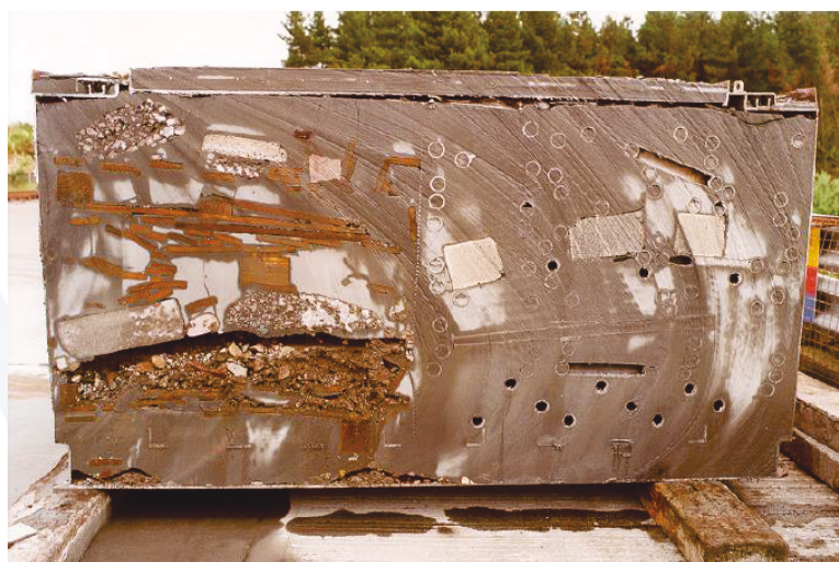
Figure 14. Cut-Through of Grouted Demonstration ISO Container (containing encapsulated wood, rubble, concrete blocks and metal pipes) (Ref 246).
