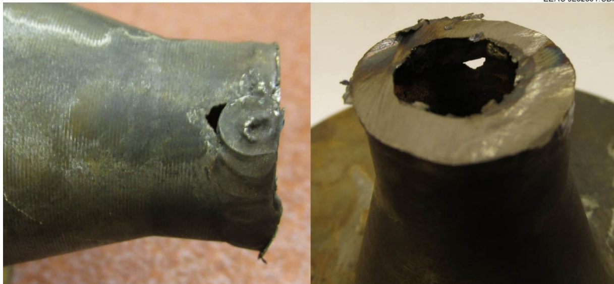
Figure 4-19. Corrosion of carbon steel flange.
