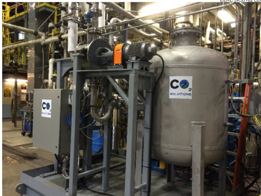
Figure 2-2. Photo of the RPB system provided by CO 2 Solutions.
