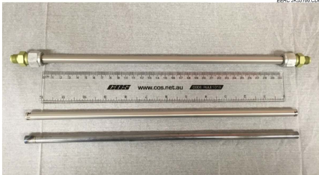
Figure 3-11. Example of as-received tube (bottom), Pd-coated separator (middle), and a separator sealed with compression fittings (top).
