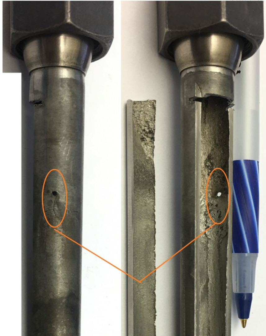
Figure 4-20. Air-cooled heat exchanger corrosion and pinhole (interior and exterior).
