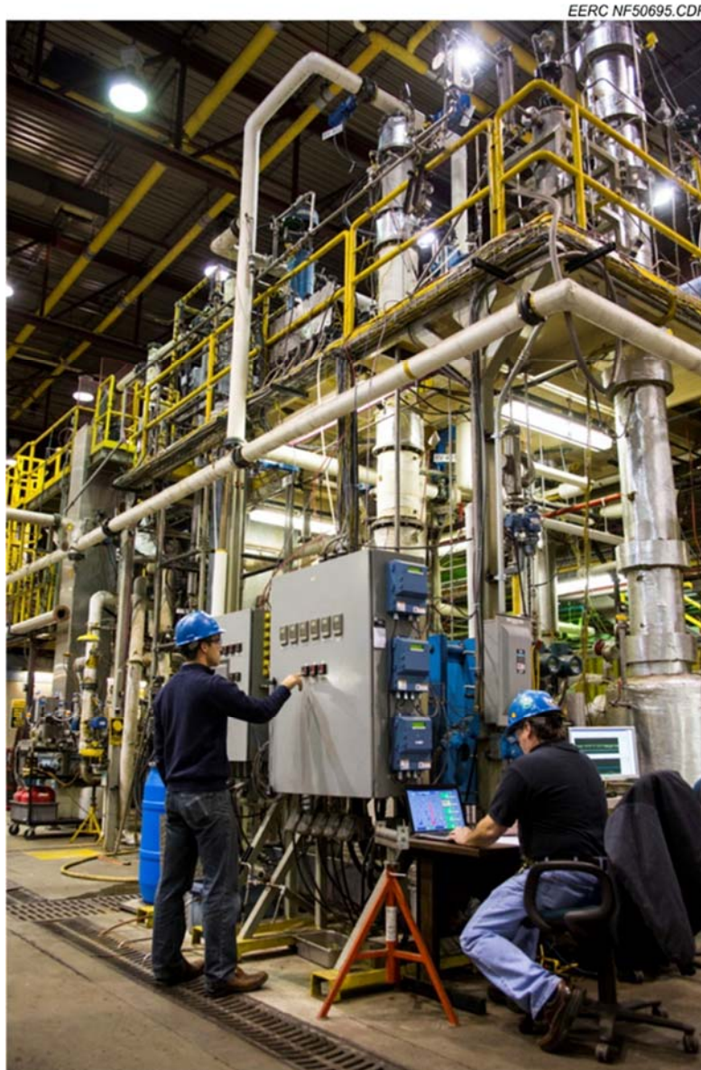
Figure 2-1. EERC solvent-based capture system and control station.
