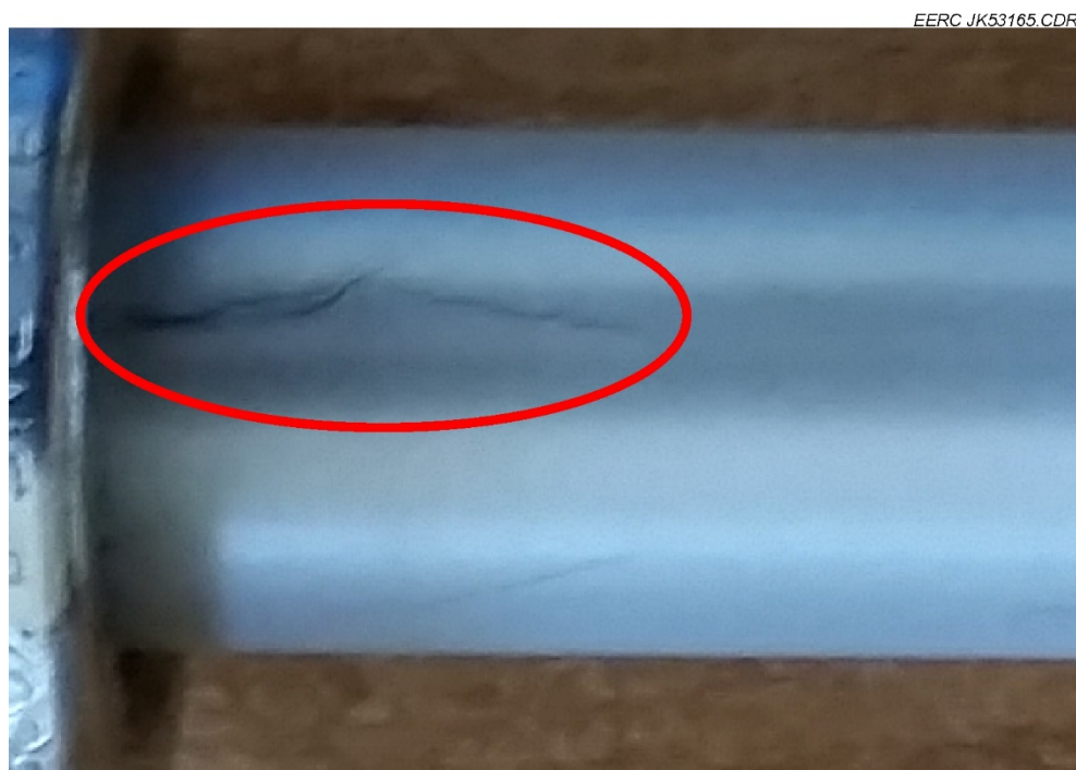
Figure 3-24. Crack in Separator 268.
