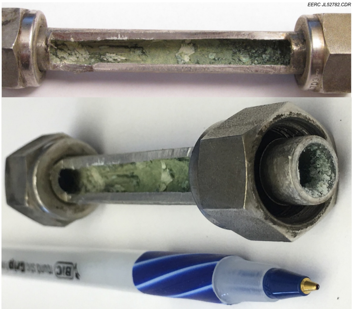
Figure 4-21. Internal deposit formation in water recirculation tubing.
