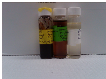
Figure 39. Product sample from SCF methanol with cellulose at 300°C
