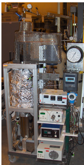
Figure 47. High-pressure 316 stainless-steel batch reactor
