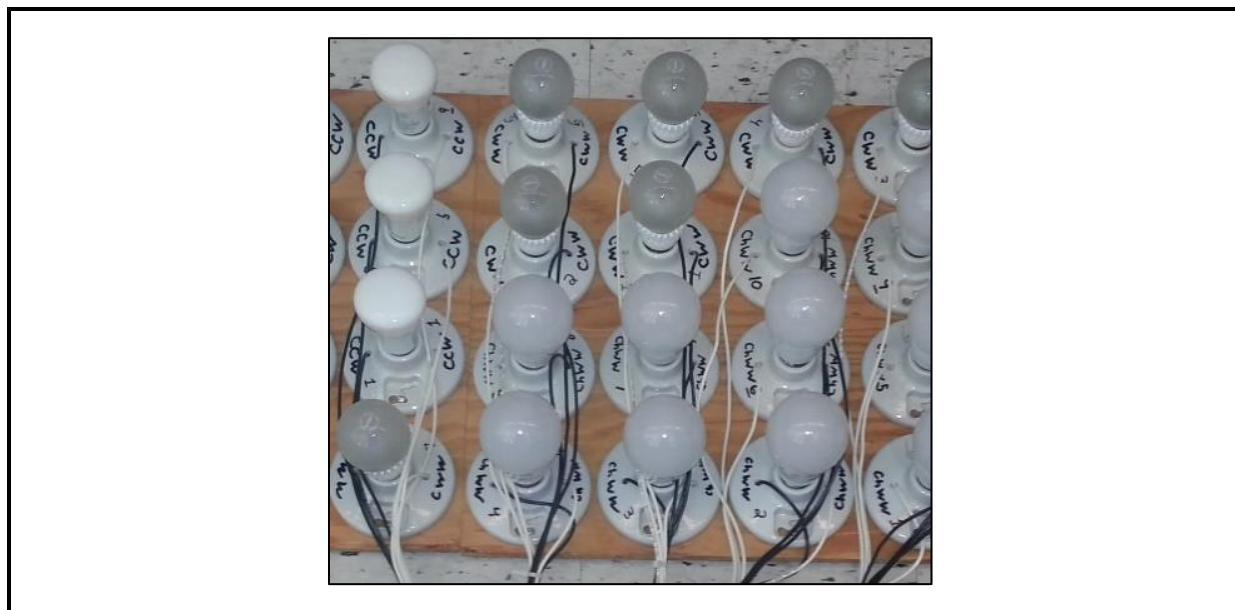
Figure 4C-8. Photo of the Configuration of A19 Lamps during the SSL1 and SSL2 Testing Protocols
