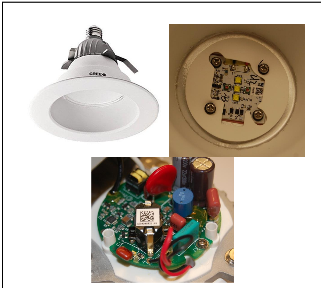
Figure 4D-23. Picture of the Cree CR6 Downlight and Driver (left) and Hybrid LED Light Engine (right)
