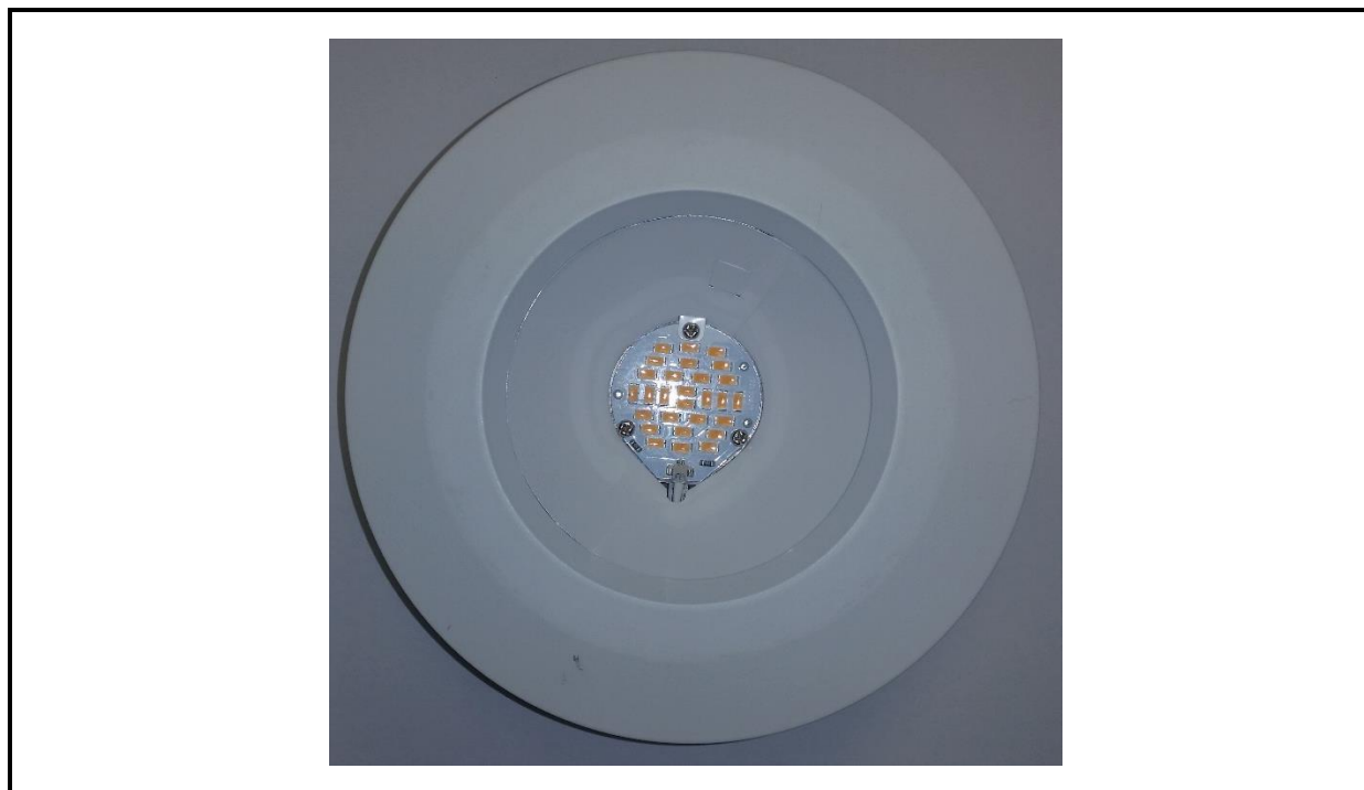
Figure 4D-49. Picture of the Commercial Electric T-65 6" Luminaire With the Front Lens Removed
