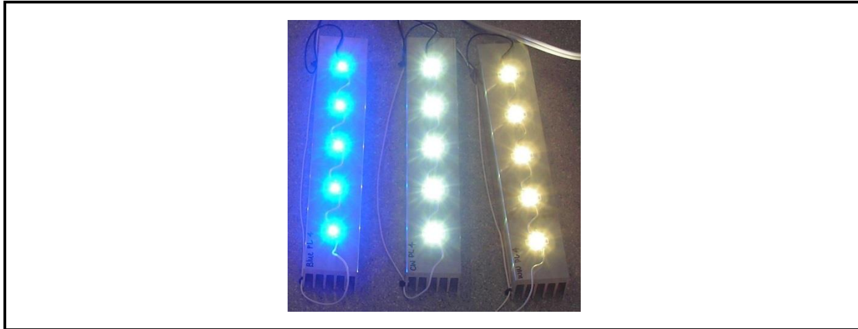
Figure 4B-7. Image of the Mounting Configuration Used for Testing Individual LEDs
