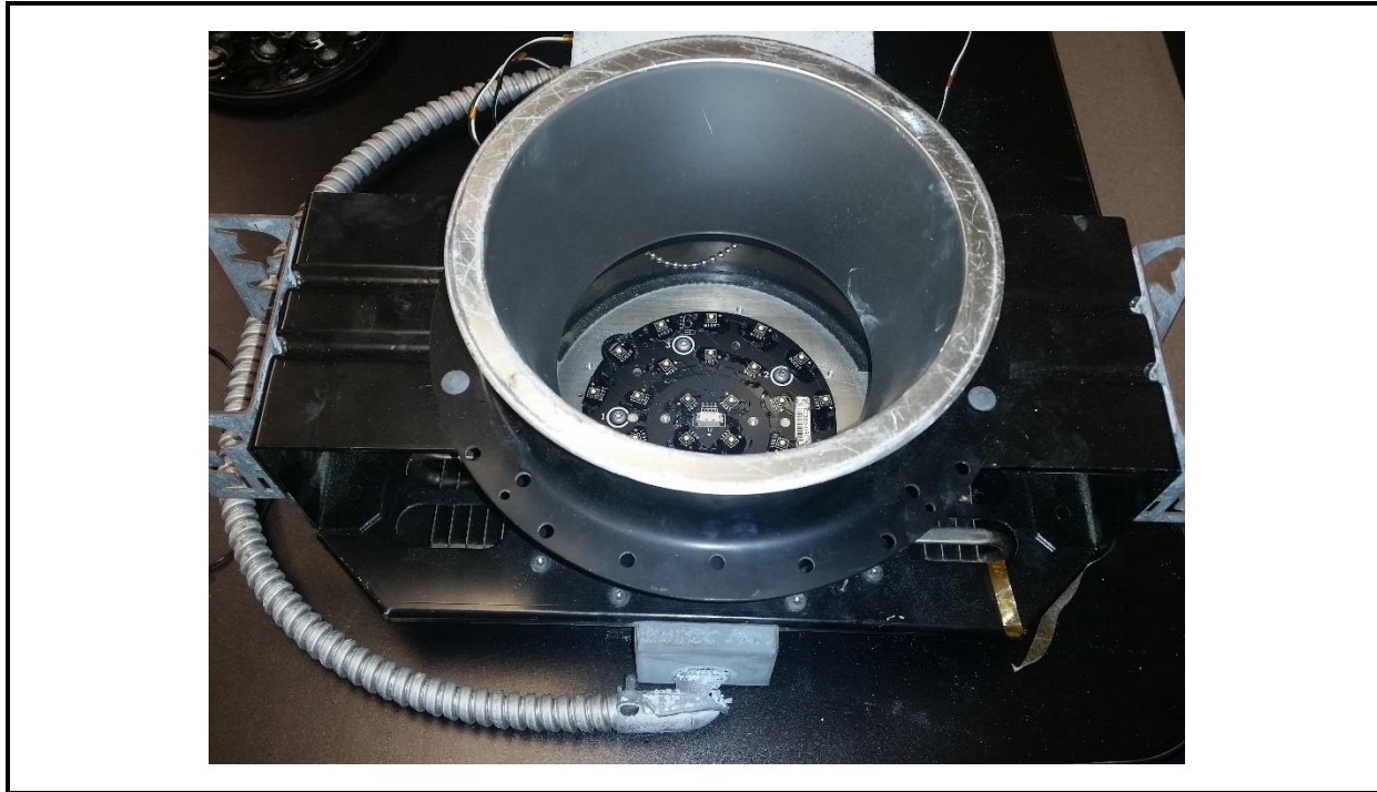
Figure 4D-36. Picture of Cree Essentia Luminaire Subjected to 8585 Testing by RTI
