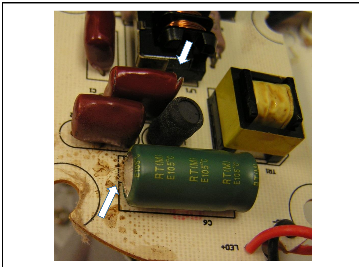
Figure 4D-69. Driver for 6" Downlight that Exhibited Multi-component Failure
