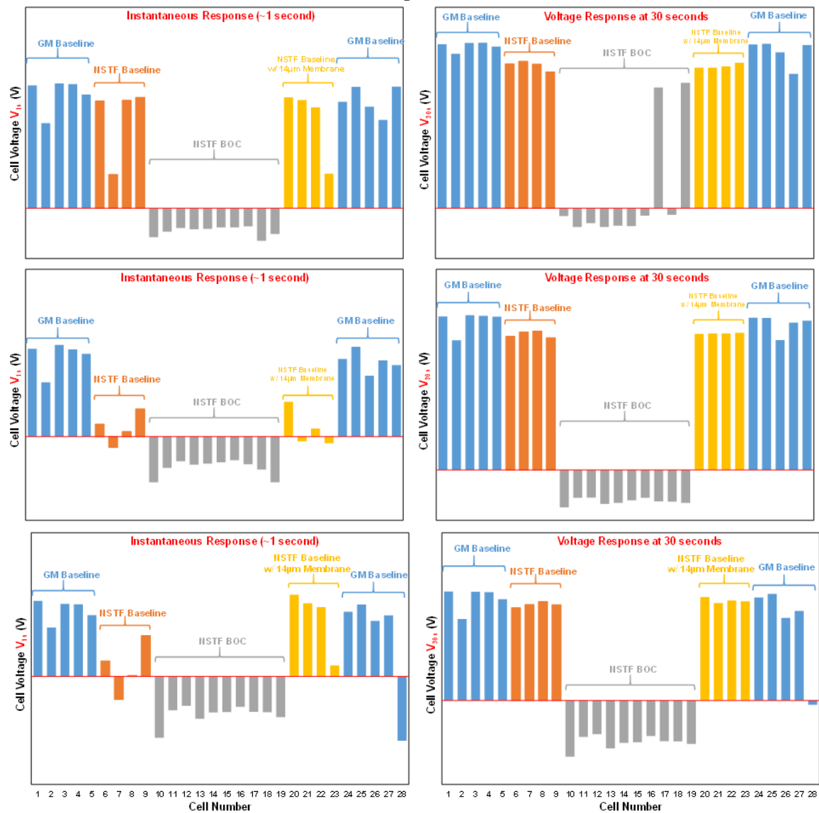
Figure 196. Stack Load Transients at 70C, 100% RH; 50C, 0% RH; and 40C, 0% RH (top to bottom). Left: Instantaneous. Right: After 30s.
