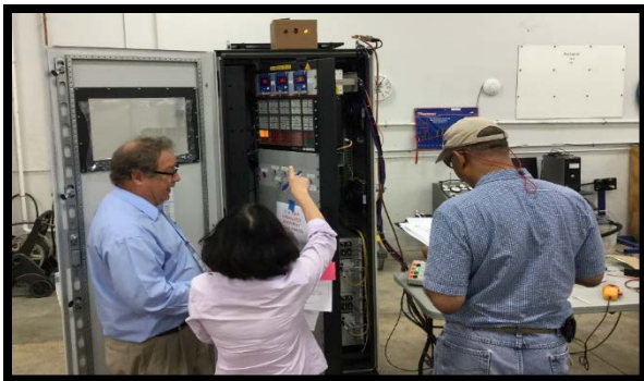
CAS CIDAS Panel Factory Acceptance Test
