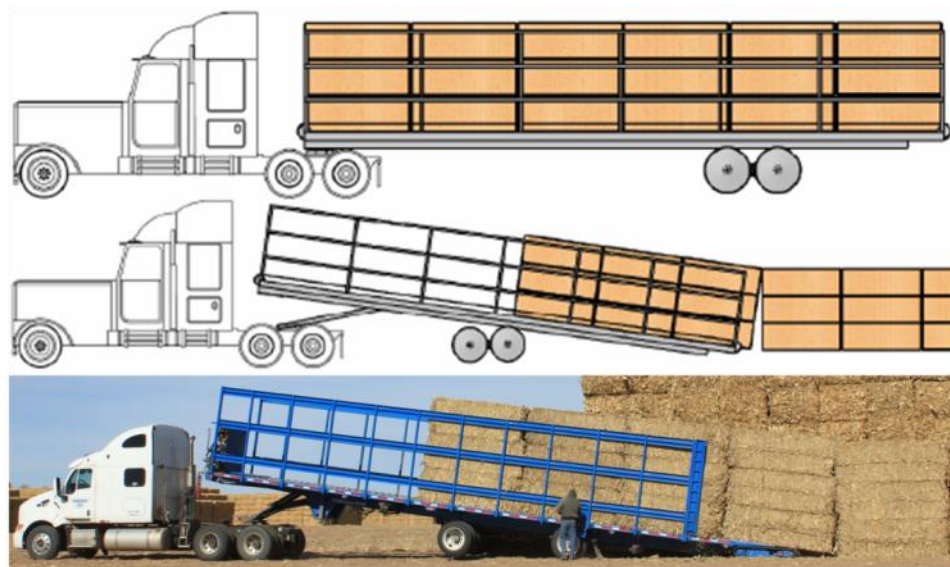
Figure 10 – Self Loading Trailer Concept Design to Finished Prototype, designed in 2010
