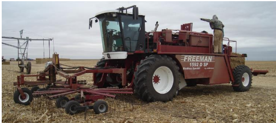
Figure 5 – Kelderman Self Propelled Baler with Front-mounted Miller Tedder Rake
