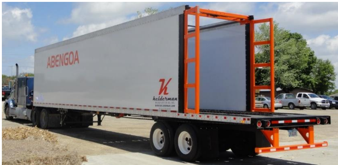
Figure 15 – 3 rd Generation Self Loading Trailer, designed in 2013
