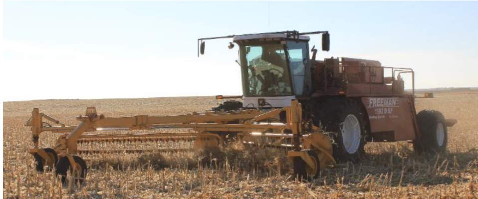
Figure 4 – Kelderman Self Propelled Baler with Front-mounted Vermeer R2800 Basket Rake
