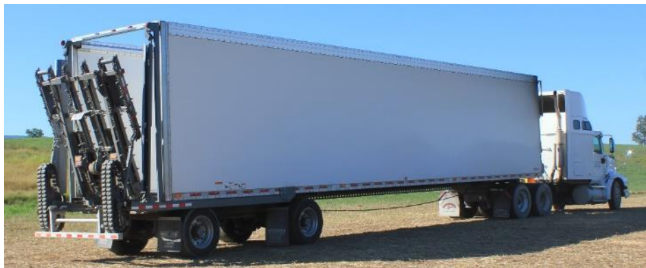
Figure 14 – 2 nd Generation Self Loading Trailer in Transport Mode
