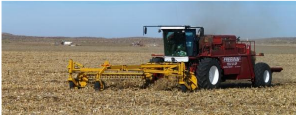
Figure 57 – Self Propelled Baler with Front-mounted Basket Rake
