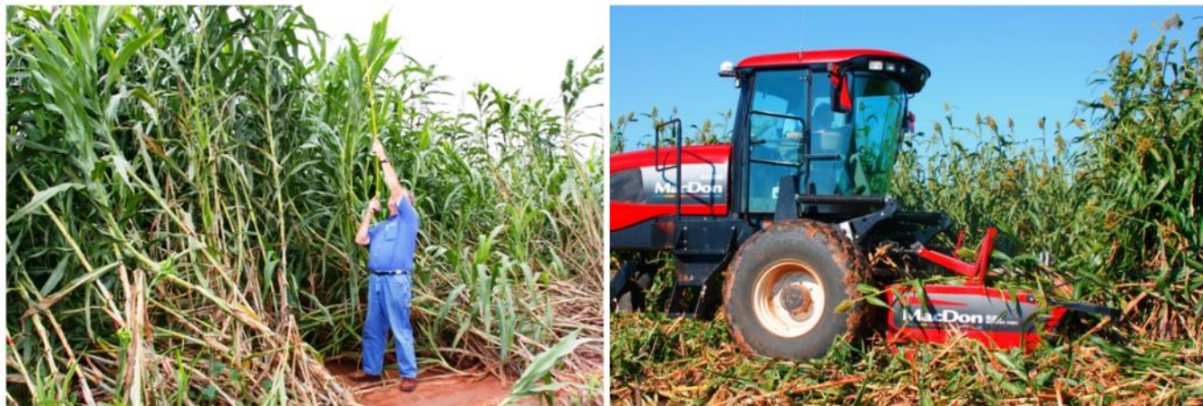
Figure 18 – MacDon Conventional Windrower Attempting to Windrow 20' Tall Energy Sorghum
