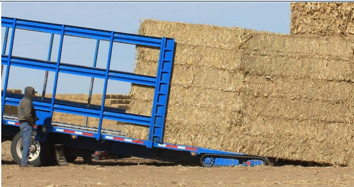
Figure 11 – Close-up View of the Loading/Unloading Mechanism
