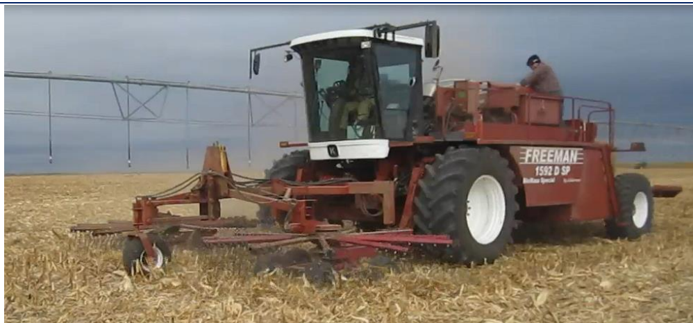
Figure 58 – Self Propelled Baler with Front-mounted Tedder Rake
