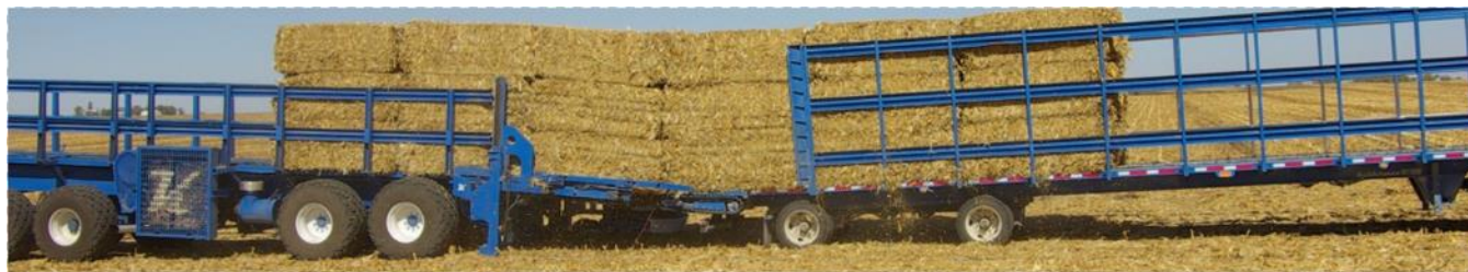
Figure 16 – Direct Transfer of a Module of Bales from the BPT to a SLT
