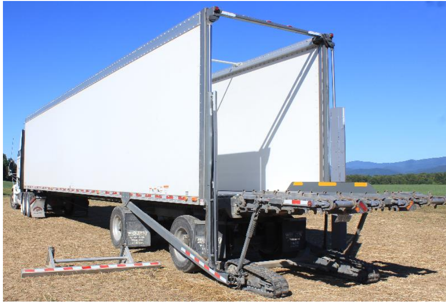
Figure 13 – 2 nd Generation Self Loading Trailer, designed in 2012
