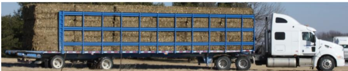
Figure 12 – 1 st Generation Self Loading Trailer with a Full Load
