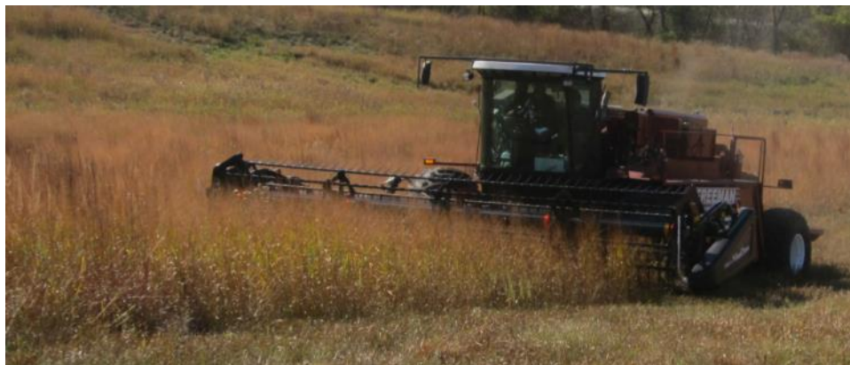
Figure 3 – Kelderman Self Propelled Baler with Front-mounted MacDon Draper Header
