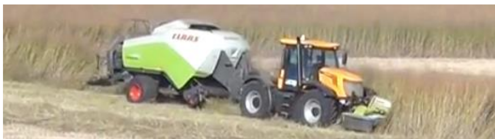
Figure 65 – FDCE Harvesting WSG in a Single Pass with a Claas 3300 Square Baler
