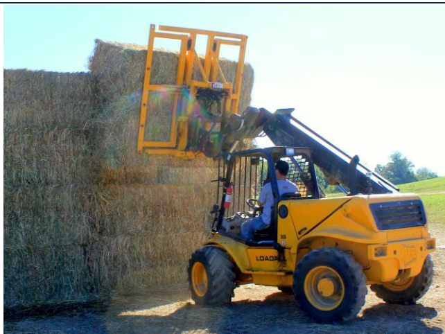
Figure 53 – Telehandler in Operation
