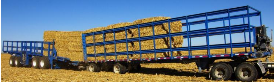
Figure 62 – Direct Transfer of Bales from BPT to SLT
