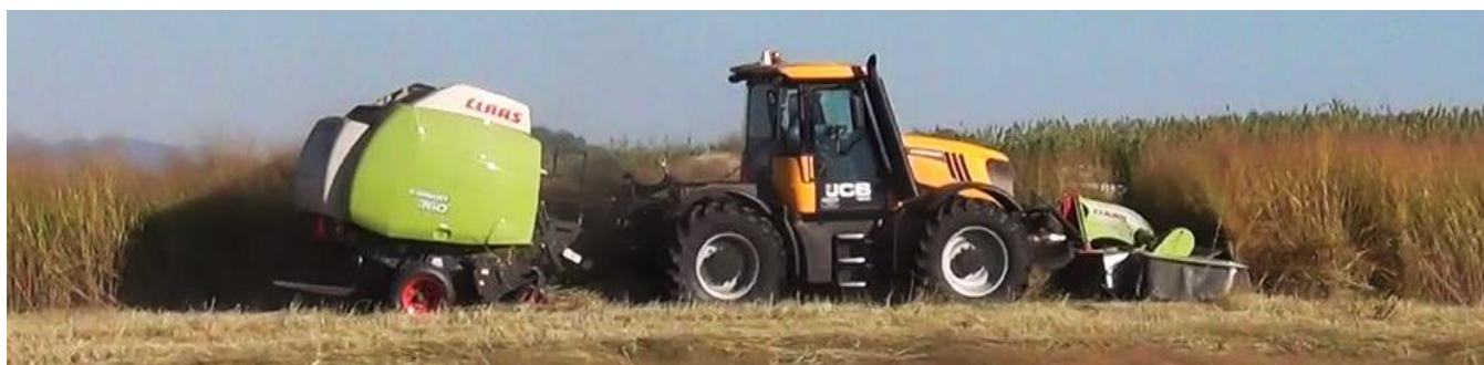
Figure 64 – FDCE Harvesting WSG in a Single Pass with a Claas 360 Round Baler
