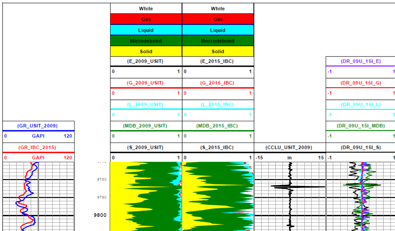
Figure 42 Comparison of ultrasonic data collected at 9800 ft in CFU31F-2. Note the 2009 data are denoted with USIT and the 2015 data are denoted with IBC.
