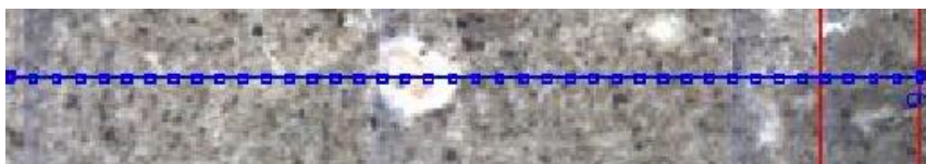
Figure 23 LA-ICP-MS Line 1 results across the sample collected in CFU31-F2 at 7900 ft showing Ca/Si, Ca/Al, and Ca/Fe mole ratios.
