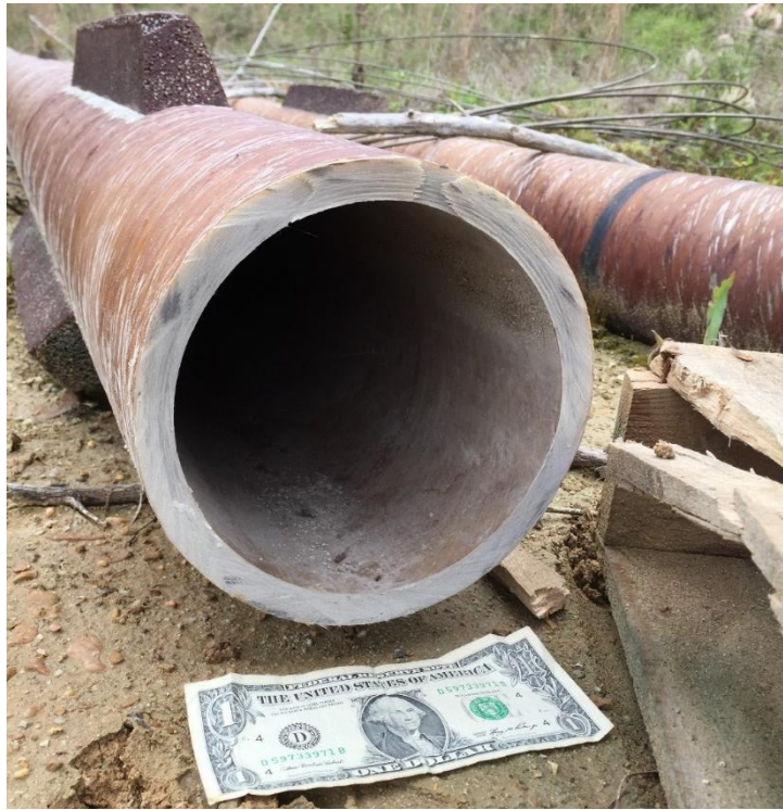
Figure 4 Bluebox 2500 casing used to construct both monitoring wells.
