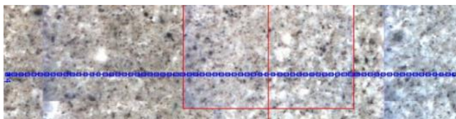
Figure 66 LA-ICP-MS Line 9 results across the sample collected in CFU31-F2 at 9800 ft showing Ca/Si, Ca/Al, and Ca/Fe mole ratios.
