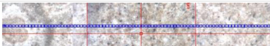
Figure 192 LA-ICP-MS Line 4 results across the sample collected in CFU31-F3 at 10477 ft showing Ca/Si, Ca/Al, and Ca/Fe mole ratios.
