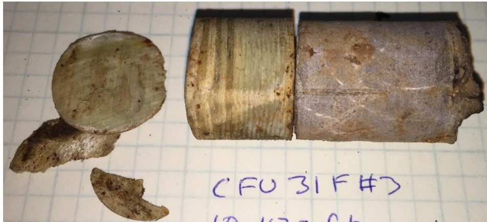
Figure 160 Sidewall core collected in CFU31-F3 at 10470 ft showing fiberglass casing on the left and cement on the left.
