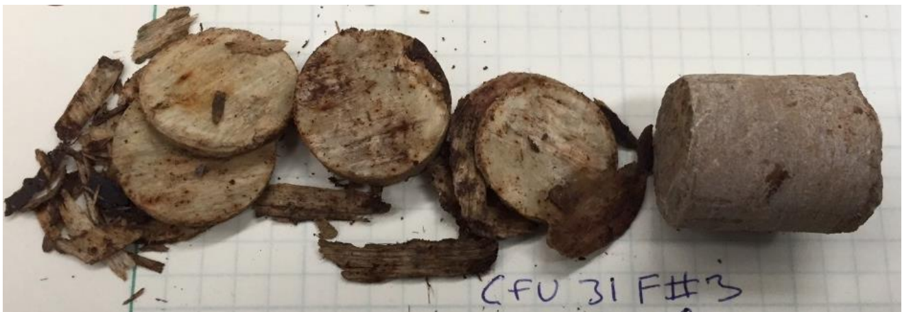
Figure 178 Sidewall core collected in CFU31-F3 at 10477 ft showing fiberglass casing on the left and cement on the left.
