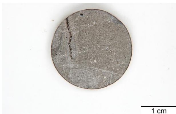
Figure 14 Section of sidewall core collected in CFU31-F2 and 7900 ft used to conduct ESEM and EDS measurement
