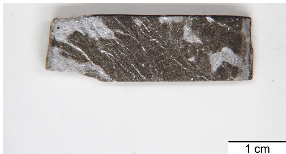
Figure 90 Portion of cement collected in CFU31-F3 at 10268 ft used for ESEM and EDS analysis.
