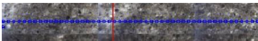
Figure 100 LA-ICP-MS Line 4 results across the sample collected in CFU31-F3 at 10268 ft showing Ca/Si, Ca/Al, and Ca/Fe mole ratios.
