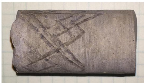
Figure 24 Sidewall core collected at 9530 ft. The casing end of the core is on the left and the formation end is on the right. Note, the sidewall core is approximately 23 mm in diameter. The jagged marks on the left half of the core are caused by reciprocation of the core bit during coring.
