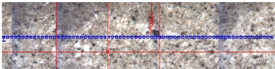
Figure 58 LA-ICP-MS Line 5 results across the sample collected in CFU31-F2 at 9800 ft showing Ca/Si, Ca/Al, and Ca/Fe mole ratios.
