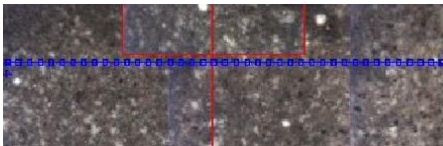
Figure 130 LA-ICP-MS Line 4 results across the sample collected in CFU31-F3 at 10380 ft showing Ca/Si, Ca/Al, and Ca/Fe mole ratios.
