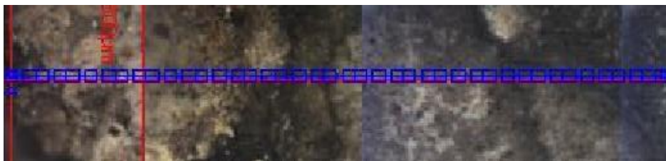
Figure 124 LA-ICP-MS Line 1 results across the sample collected in CFU31-F3 at 10380 ft showing Ca/Si, Ca/Al, and Ca/Fe mole ratios.
