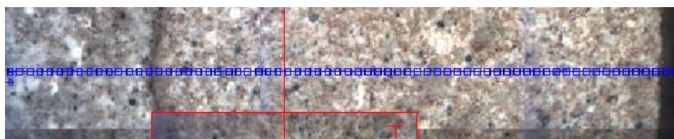
Figure 76 LA-ICP-MS Line 14 results across the sample collected in CFU31-F2 at 9800 ft showing Ca/Si, Ca/Al, and Ca/Fe mole ratios.
