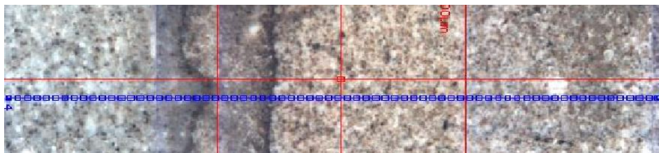
Figure 68 LA-ICP-MS Line 10 results across the sample collected in CFU31-F2 at 9800 ft showing Ca/Si, Ca/Al, and Ca/Fe mole ratios.
