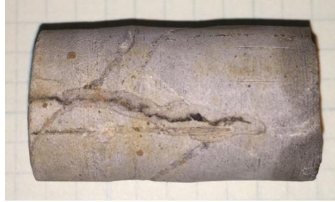
Figure 8 Sidewall core collected at 7900 ft showing crack starting at the casing end (left) and extending toward the formation end (right). Note, the sidewall core is approximately 23 mm in diameter and each square in the background is 5.08 mm on a side. It is discolored on the formation side due to exposure to hydrocarbon in the sidewall coring tool.
