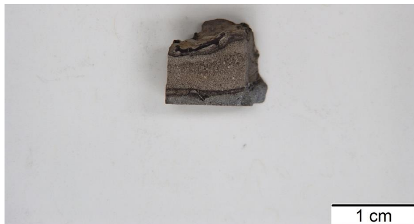
Figure 45 Photograph showing the portion of the sample collected at 9800 ft used for ESEM analyses of the formation-side reaction fronts.
