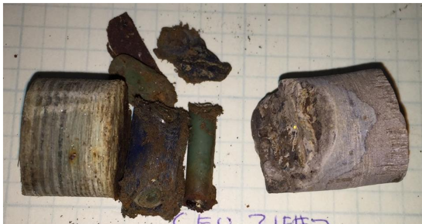
Figure 117 Sidewall core collected in CFU31-F3 showing the fiberglass casing on the left, control lines in the center, and cement on the right.
