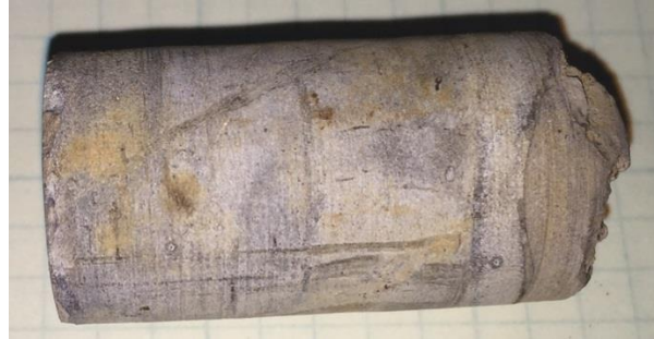
Figure 39 Sidewall core collected at 9800 ft showing a discolored zone on the formation side (right). Note, the sidewall core is approximately 23mm in diameter.
