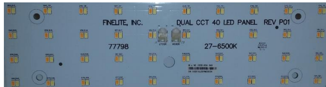
Figure 2: Picture of the tunable white MP-LED module used in this study.
