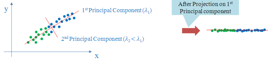
Fig. 4 – Example of dimensionality (from D = 2 to d = 1 ) reduction using PCA
