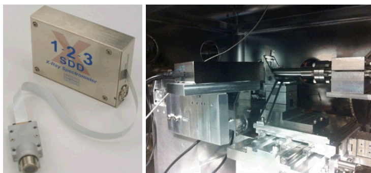
Figure 2. Left: solid state fluorescence detector (Amptek SSD) used for soft X-ray spectromicroscopy with the MES STXM. Right: mounting of the detector with respect to a STXM sample holder.
